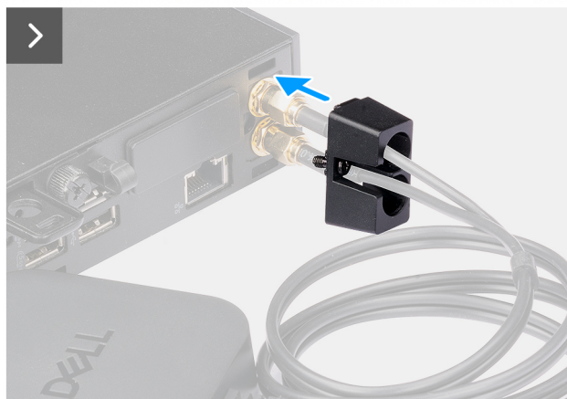
Figur 35. Installera extern puckantenn
