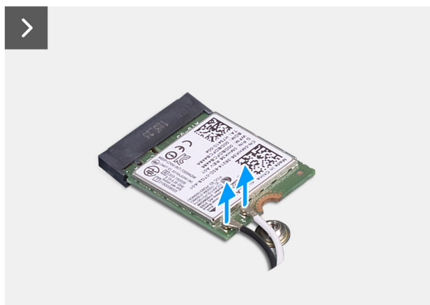
Figure 33. Removing the WLAN card
