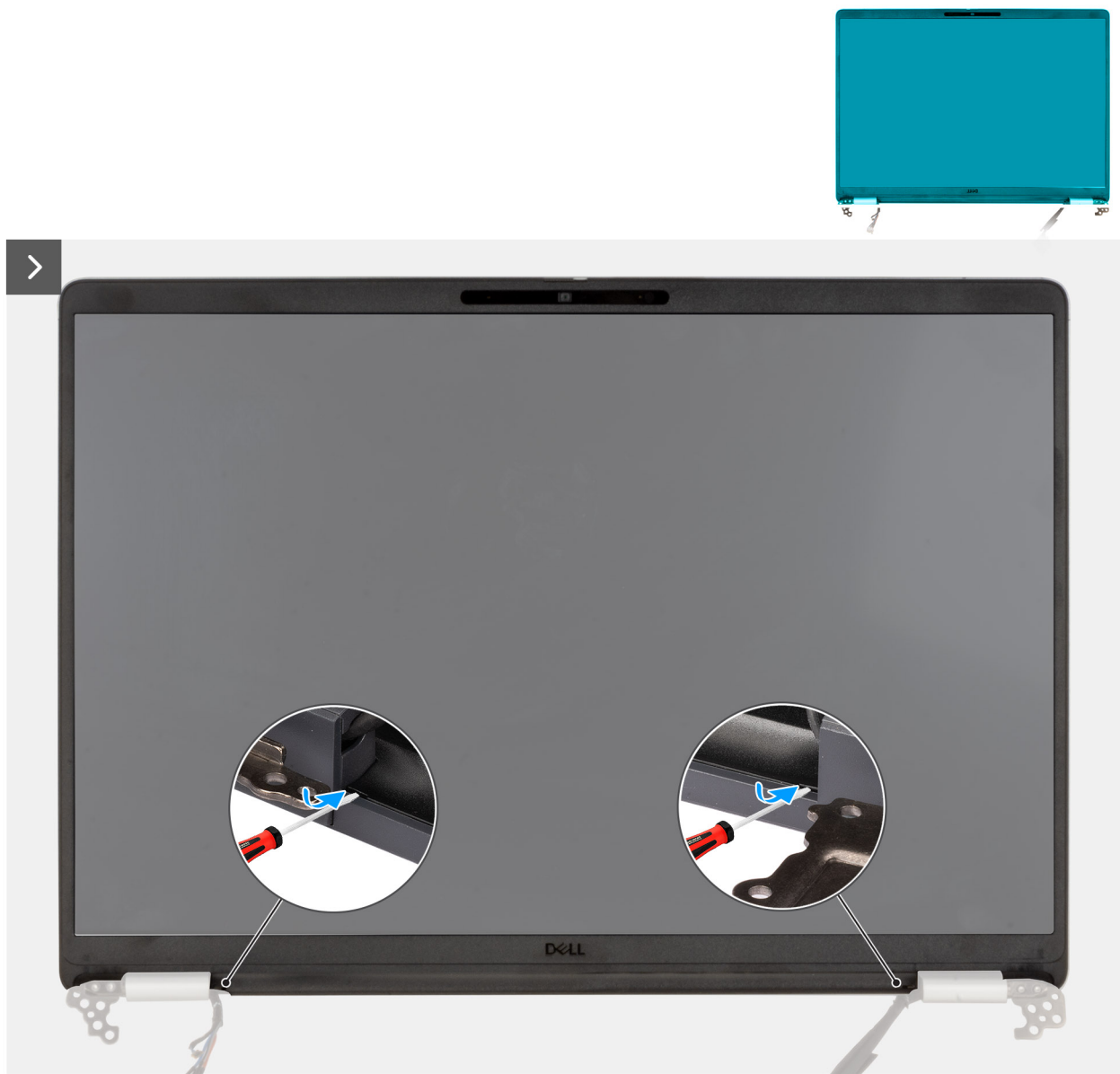
Figure 61. Prying the plastic bezel
