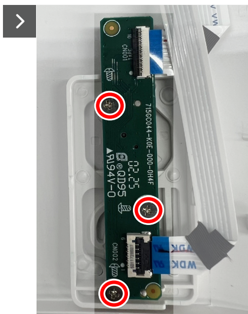
Figure 41. Removing the keypad board and disconnecting the cables
