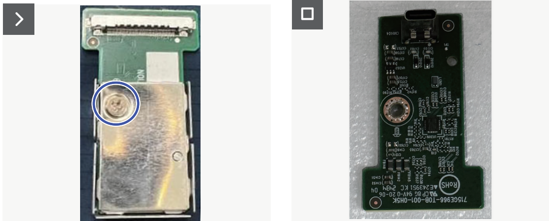
Figure 39. Removing the USB board
