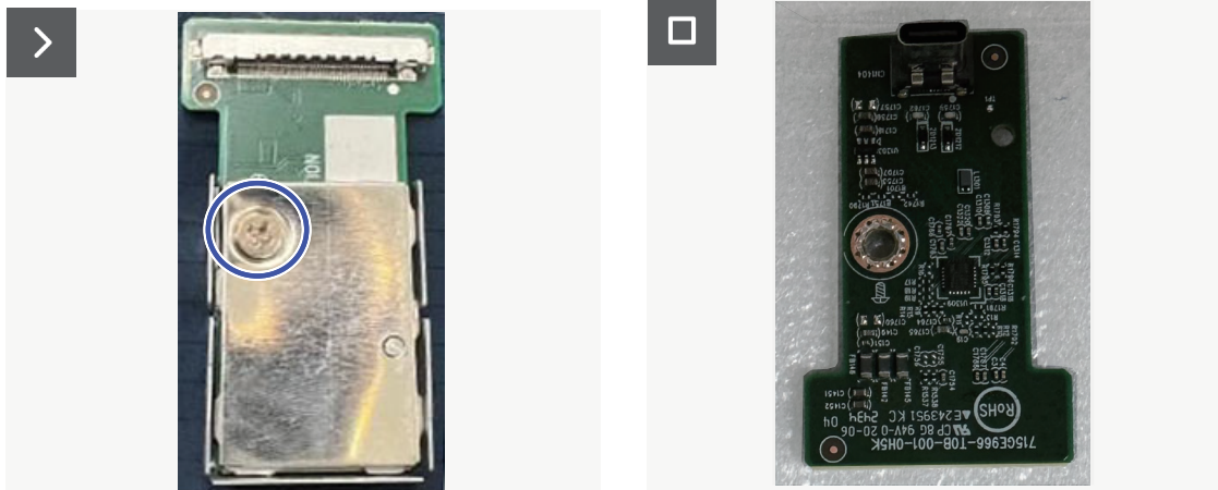
Figure 27. Removing the USB board
