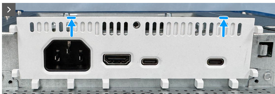
Figure 21. Replacing the metal shield I/O-cover
