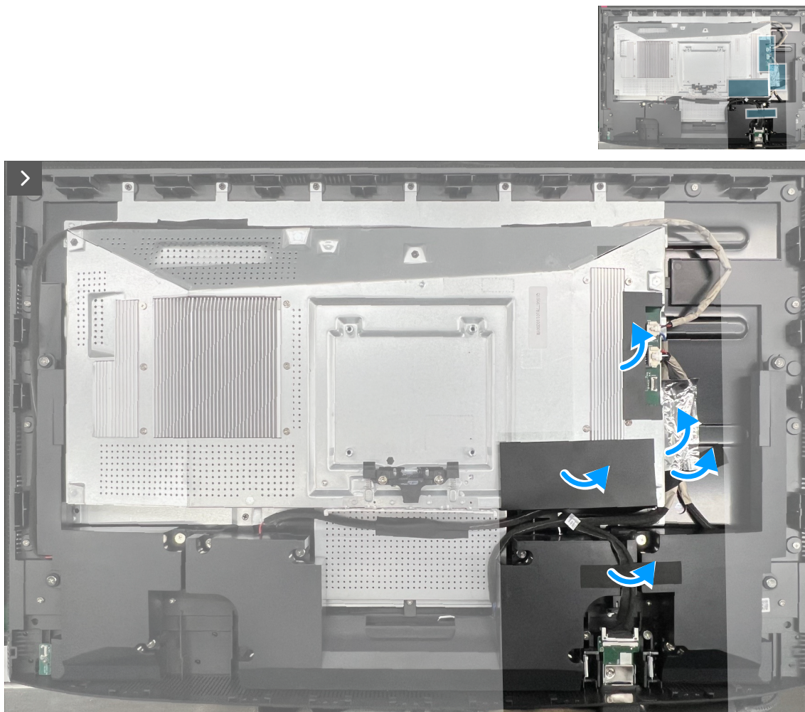
Figure 7. Peeling the tapes to secure the cables and Mylar
