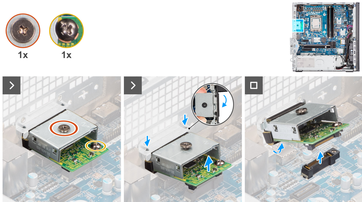
Figure 76. Removing the optional DisplayPort module
