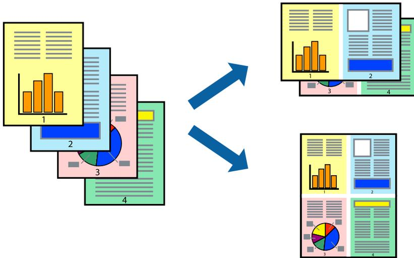
1. On the printer driver's **Main** tab, select **2-Up**, **4-Up**, **6-Up**, **8-Up**, **9-Up**, or **16-Up** as the **Multi-Page** setting.
