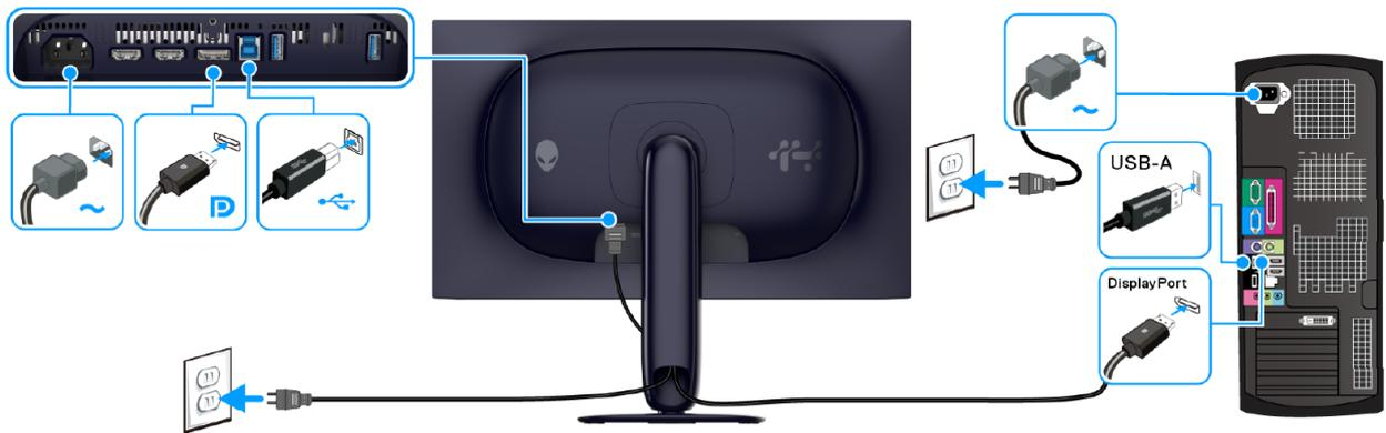
Figure 8. DisplayPort cable connection
