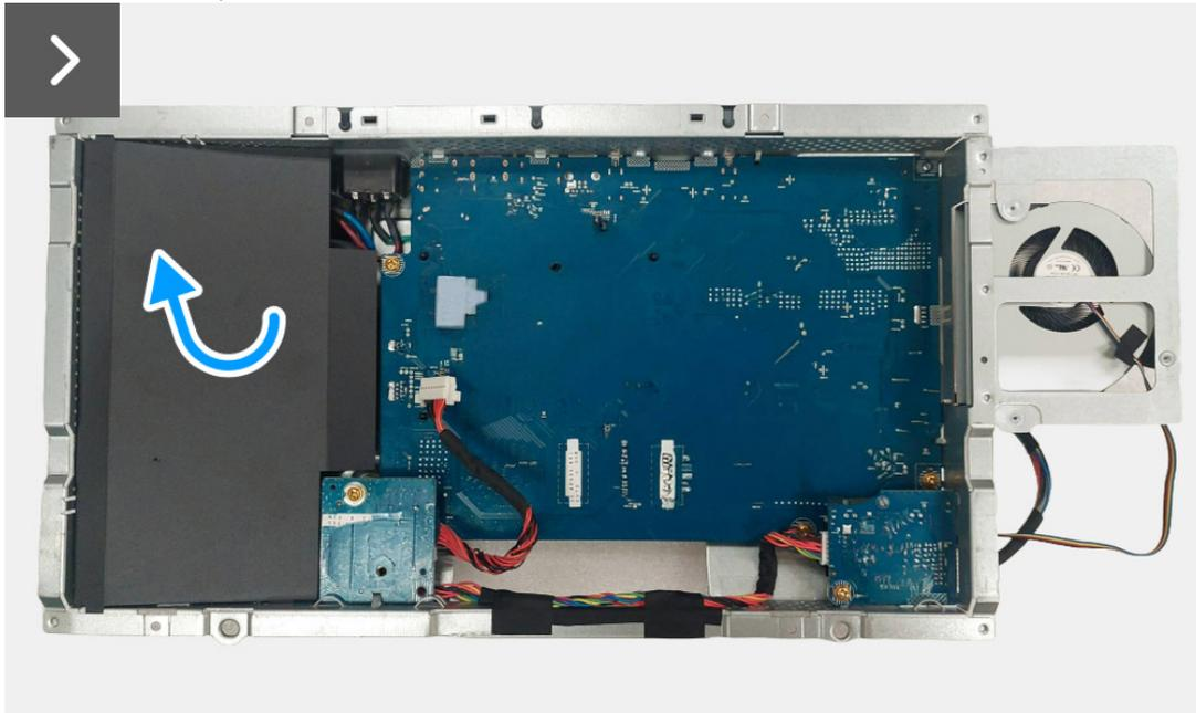
**Figure 26. Removing the switch board**
