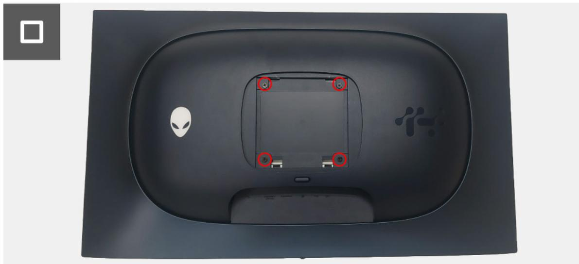
**Figure 18. Installing the back cover**
