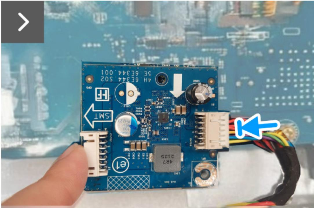
**Figure 35. Installing the DC-DC board**
