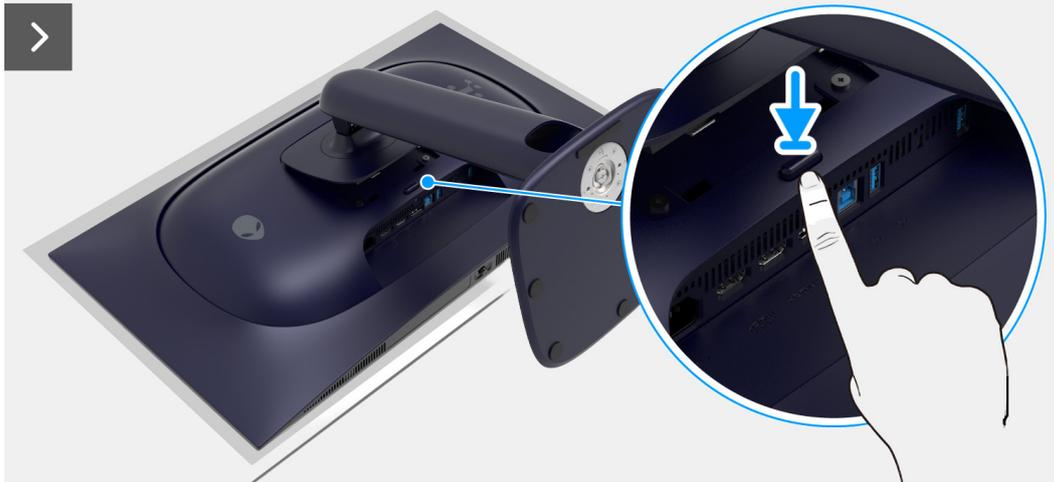
Figure 10. Removing the stand
