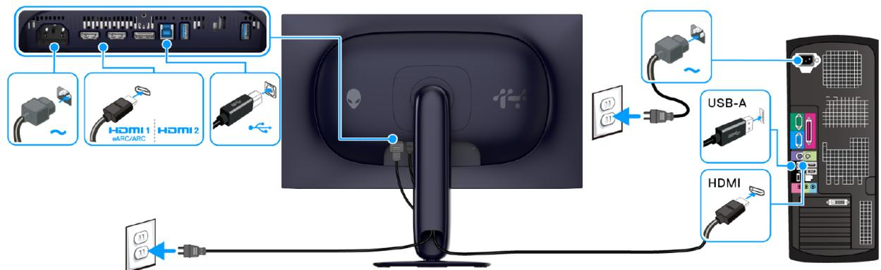
Figure 9. HDMI cable connection
