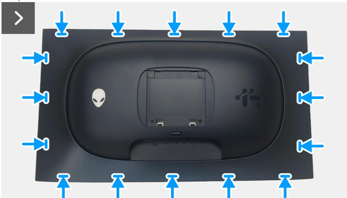
**Figure 17. Installing the back cover**
