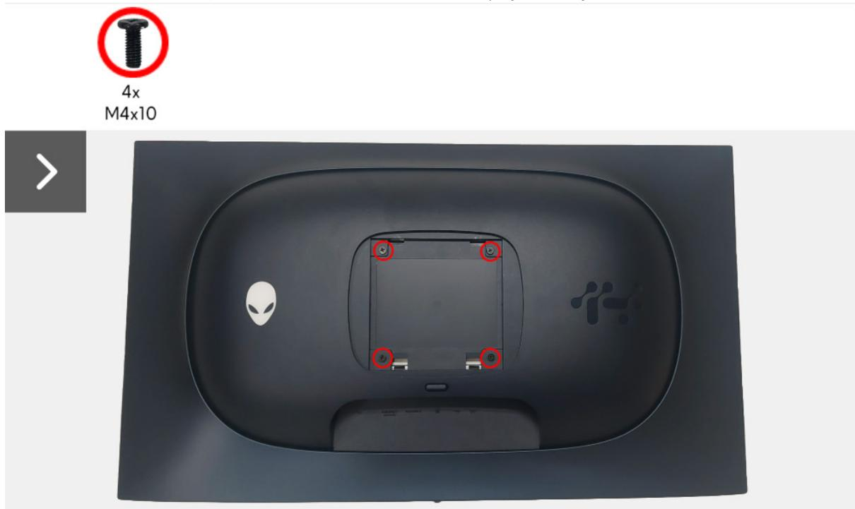
**Figure 13. Removing the back cover**
