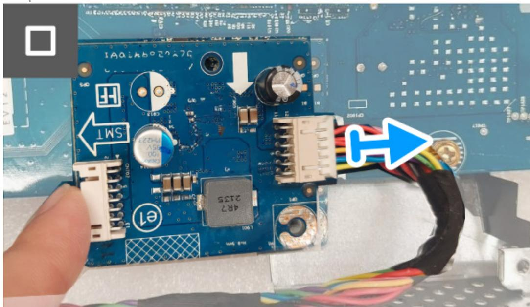
**Figure 34. Removing the DC-DC board**
