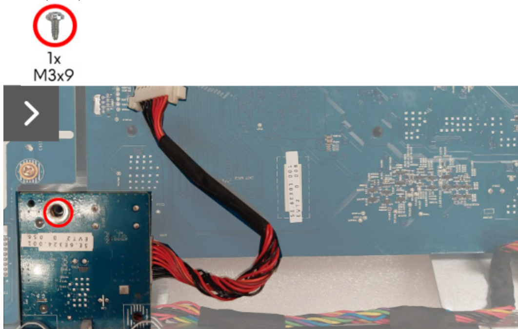
Figure 18. Removing the switch board
