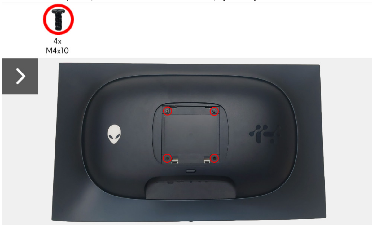
Figure 4. Removing the back cover
