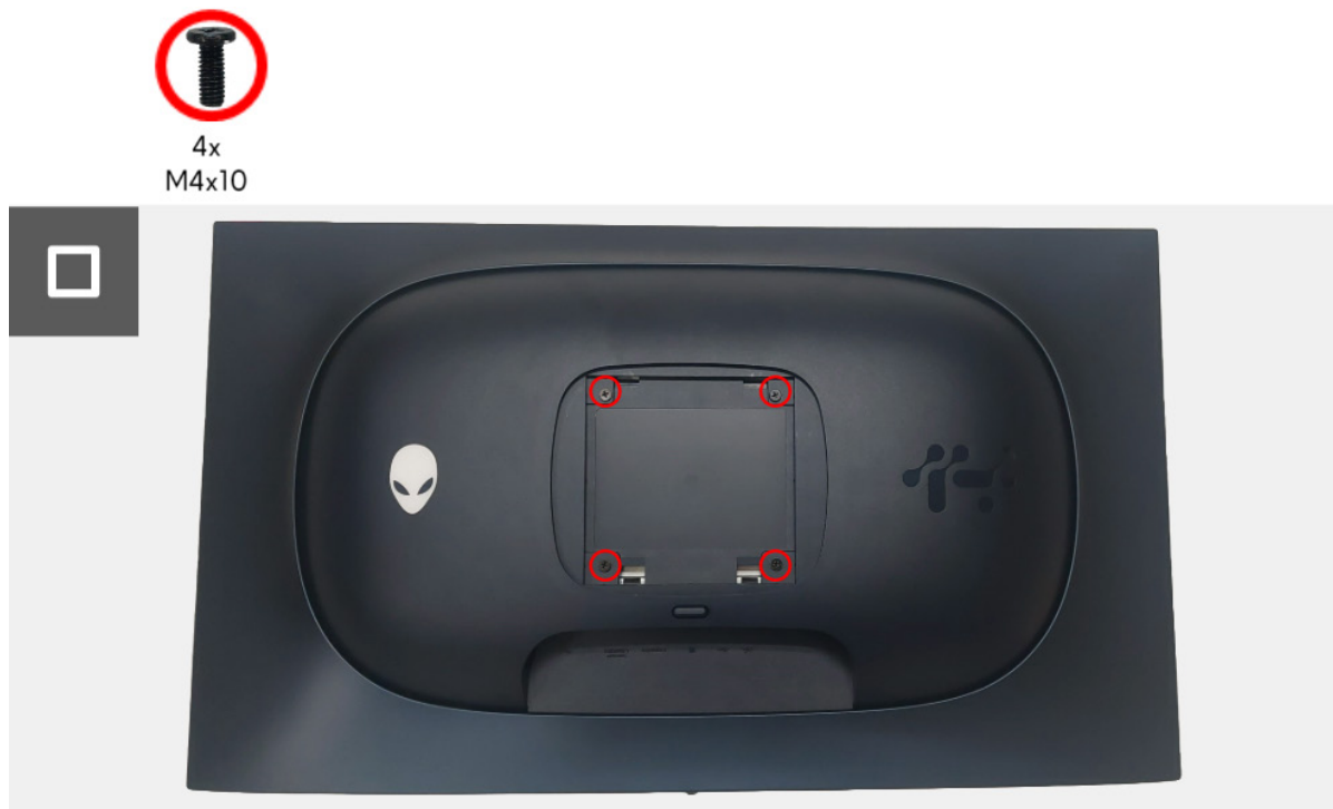
Figure 9. Installing the back cover
