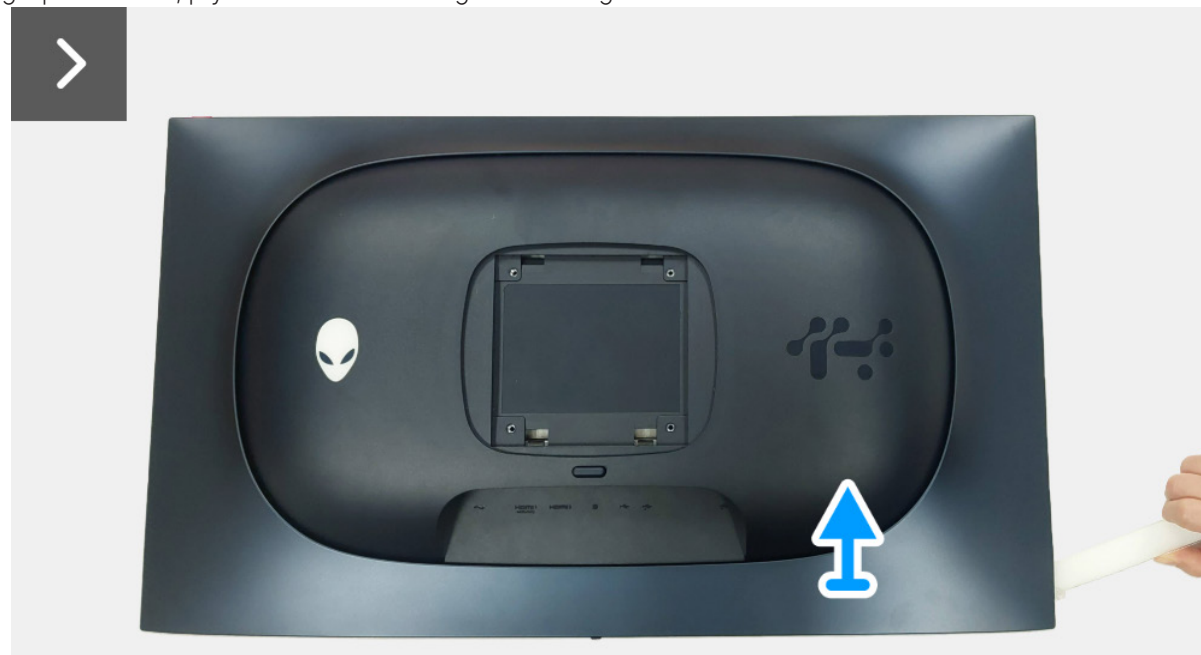
Figure 5. Removing the back cover
