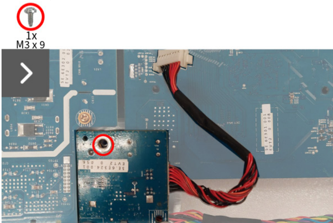
Figure 21. Installing the switch board
