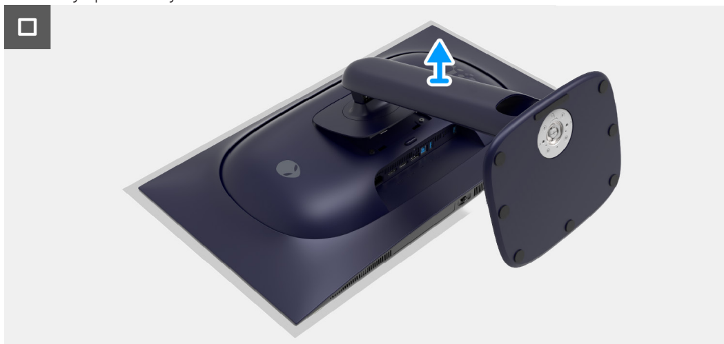
Figure 2. Removing the stand
