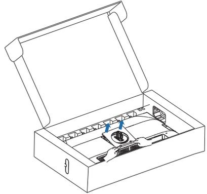
4. Loosen the assembly screws, Remove the hinge.
