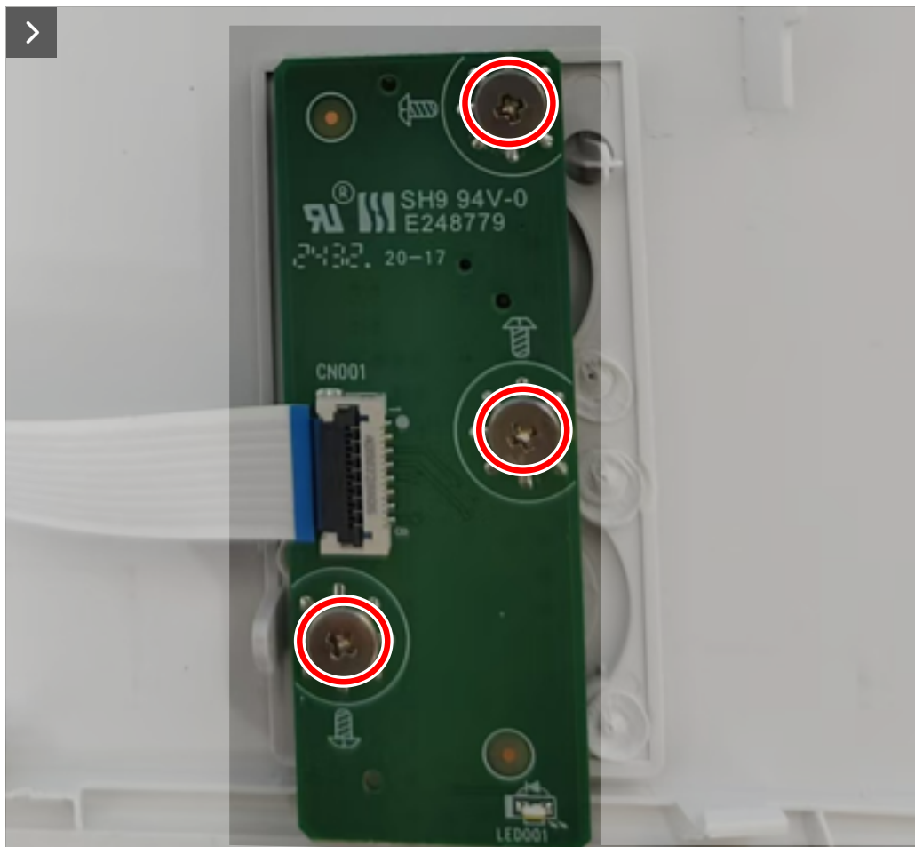
Figure 27. Removing the screws
