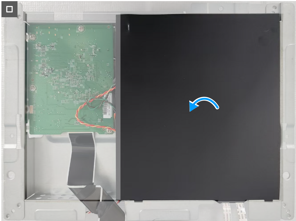
Figure 24. Placing the Mylar sheet
