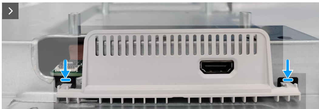
Figure 23. Replacing the metal shield I/O-cover
