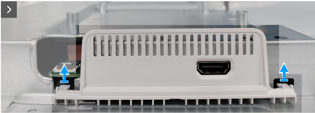
Figure 18. Removing the metal shield I/O-cover
