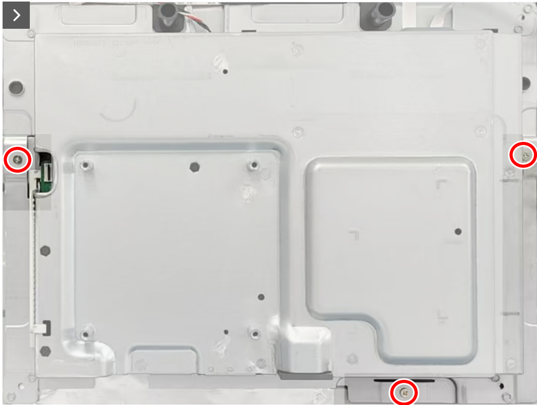
Figure 12. Removing the screws
