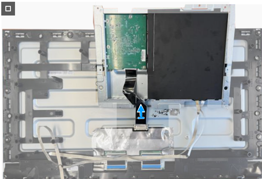
Figure 13. Disconnecting the display cable
