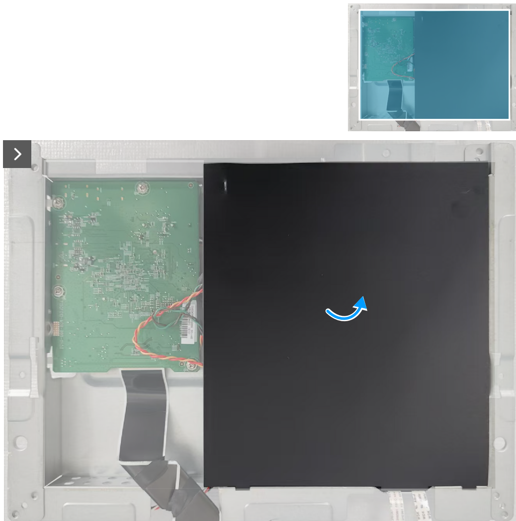
Figure 17. Removing the Mylar sheet
