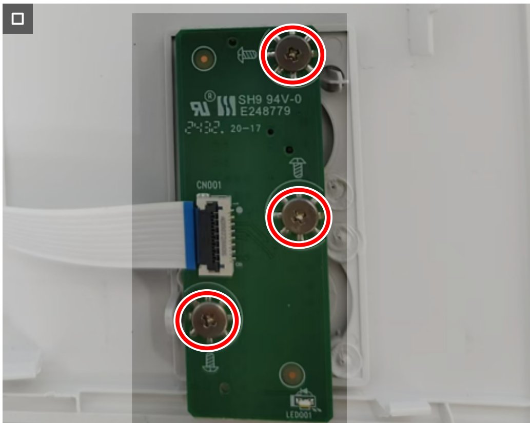
Figure 30. Replacing the screws
