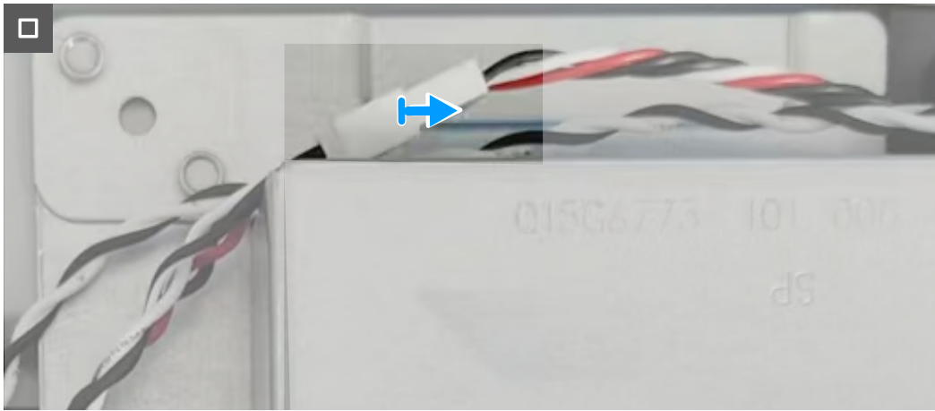
Figure 8. Disconnecting the speaker cable
