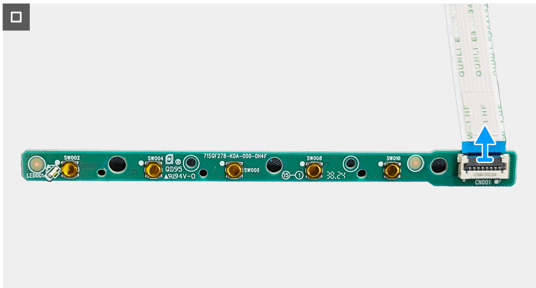
Figure 19. Removing the keypad board
