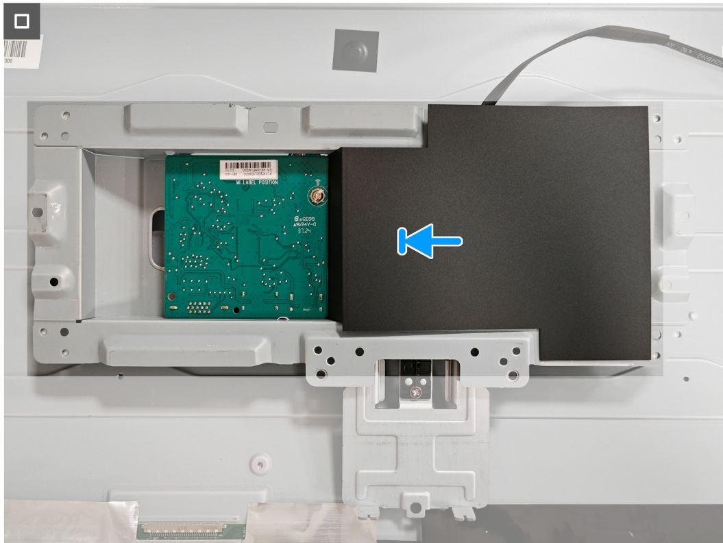
Figure 24. Installing the system board and power board
