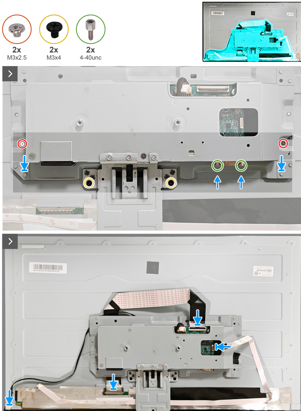
Figure 9. Installing the metal shield
