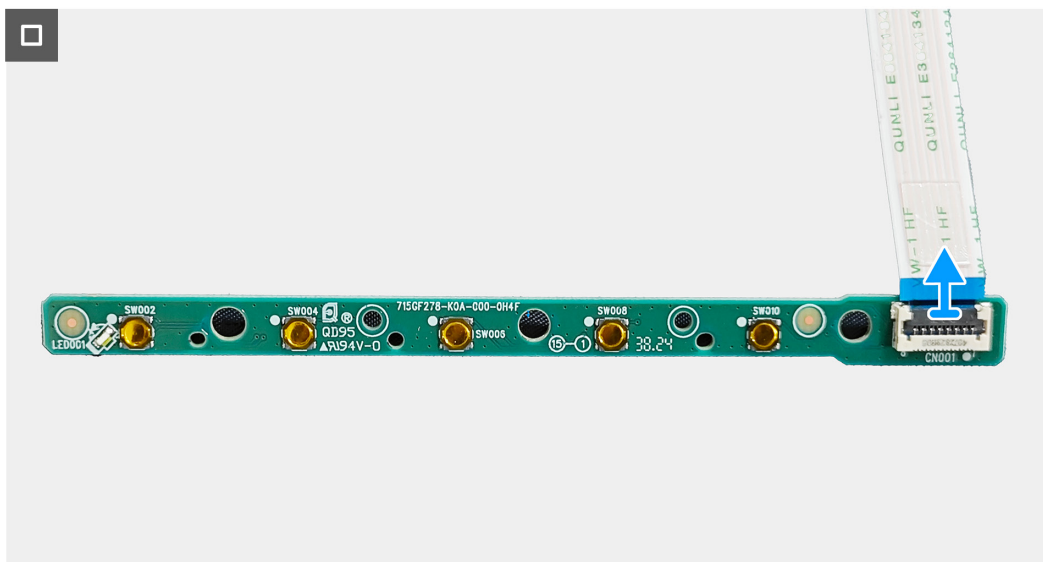
Figure 11. Removing the keypad board
