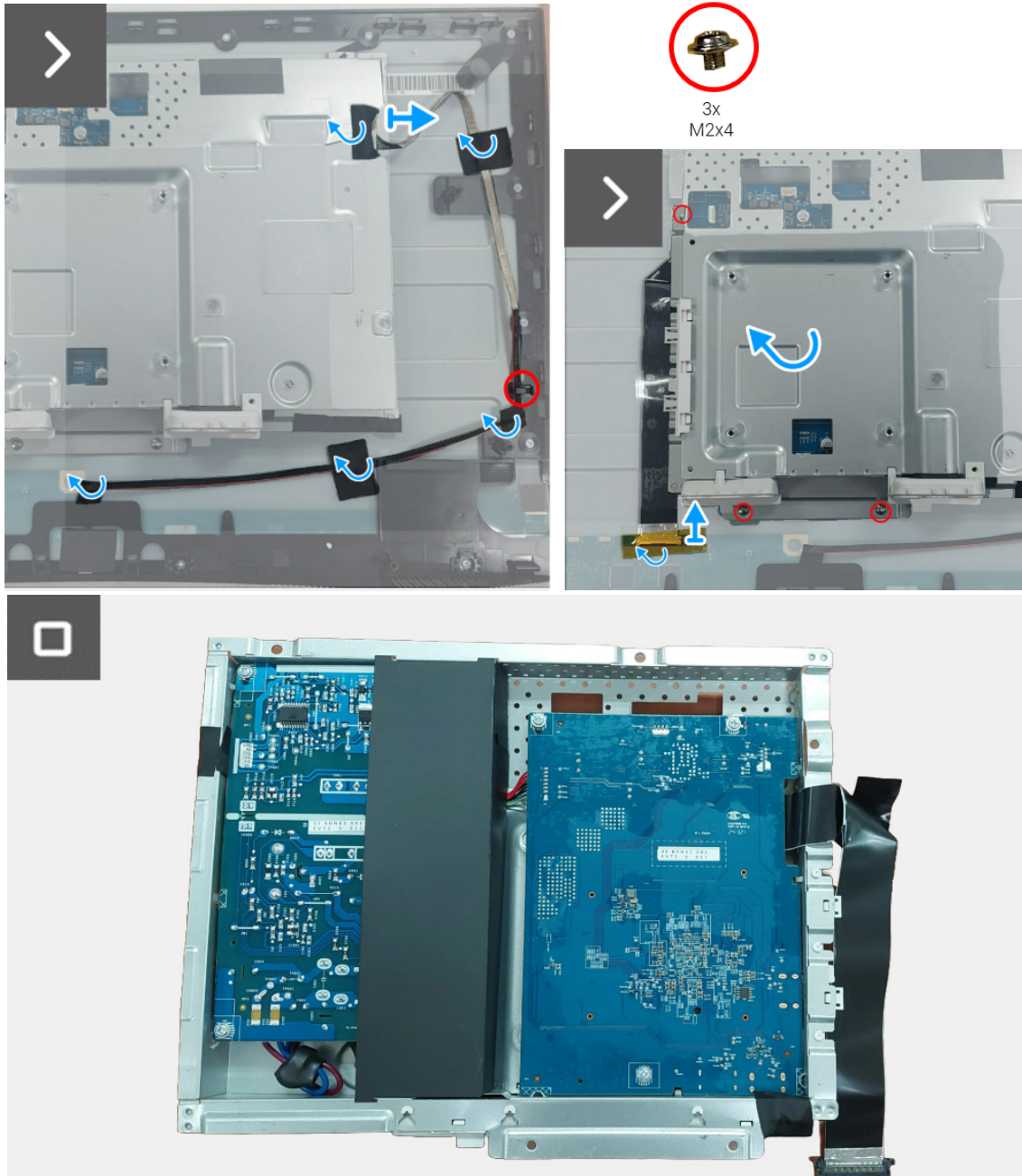
Figure 16. Removing the interface board assembly
