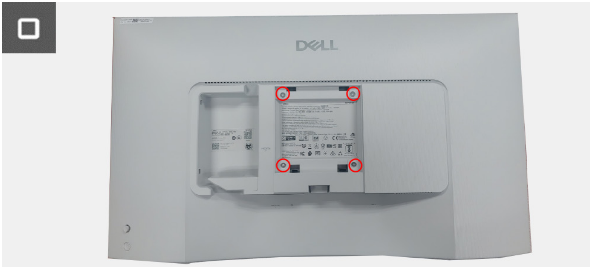
Figure 14. Installing the back cover
