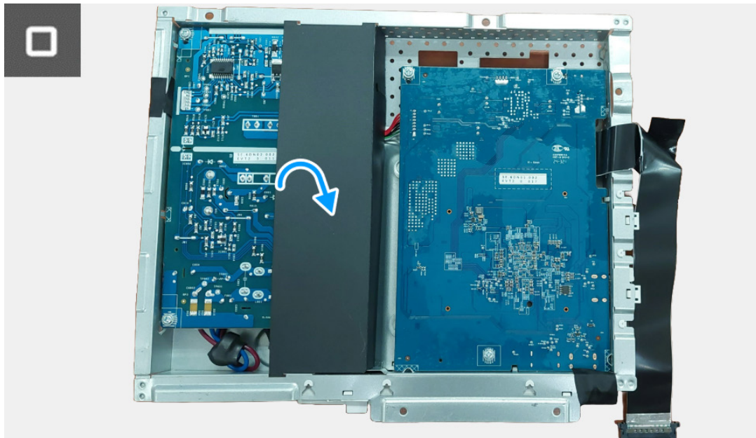
Figure 22. Installing the interface board
