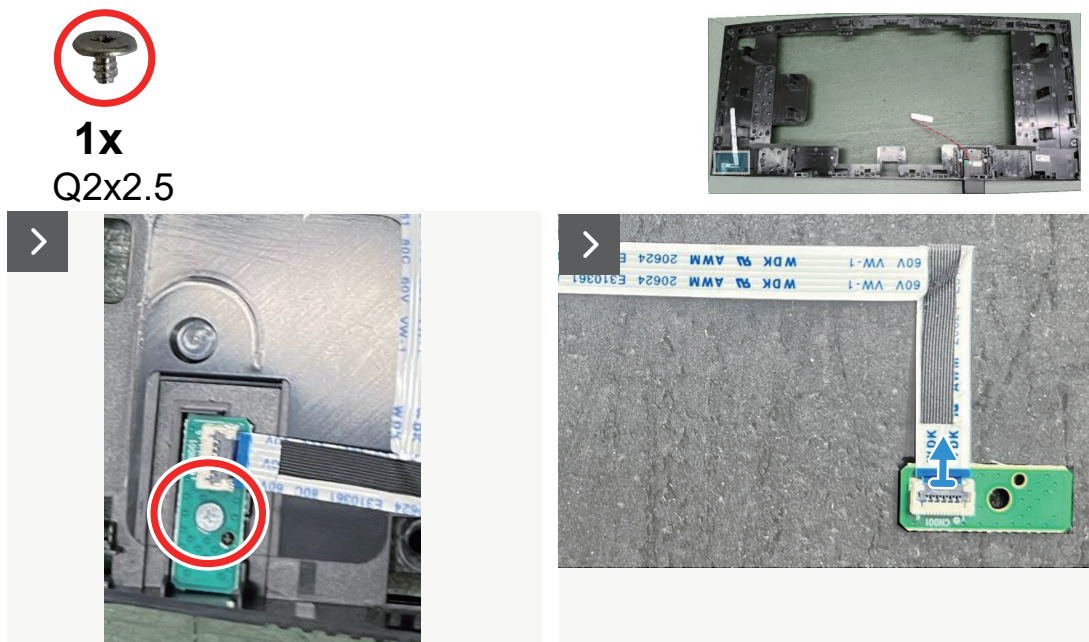
Figure 37. Removing the Lens board
