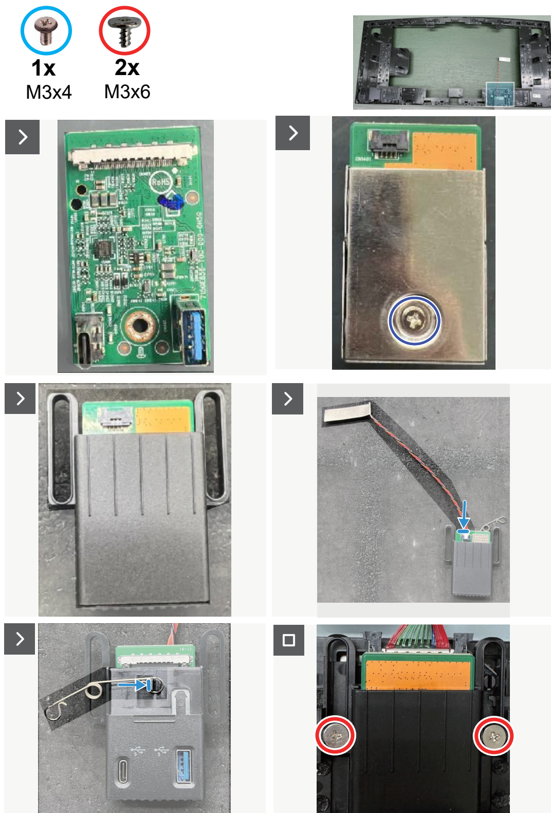
Figure 40. Installing the USB board
