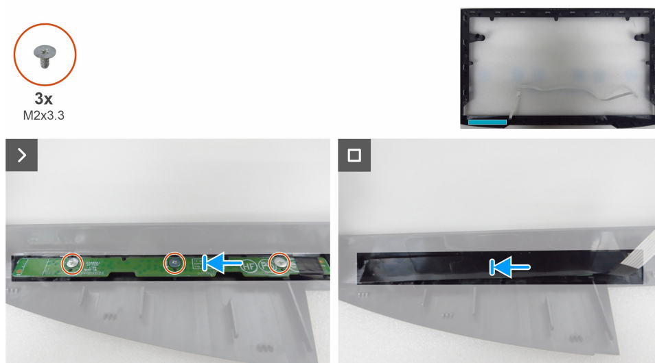
Figure 12. Installing the keypad board
