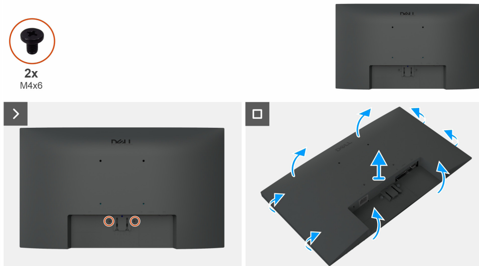
Figure 3. Removing the back cover
