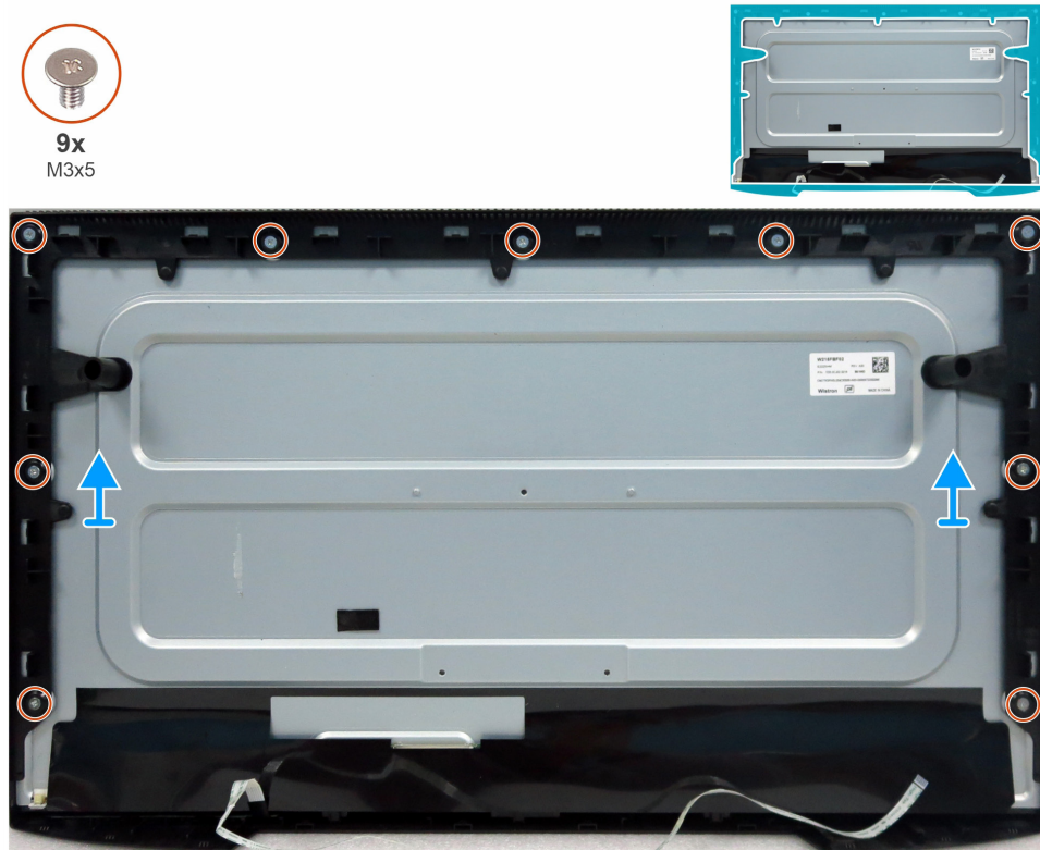
Figure 9. Removing the middle frame
