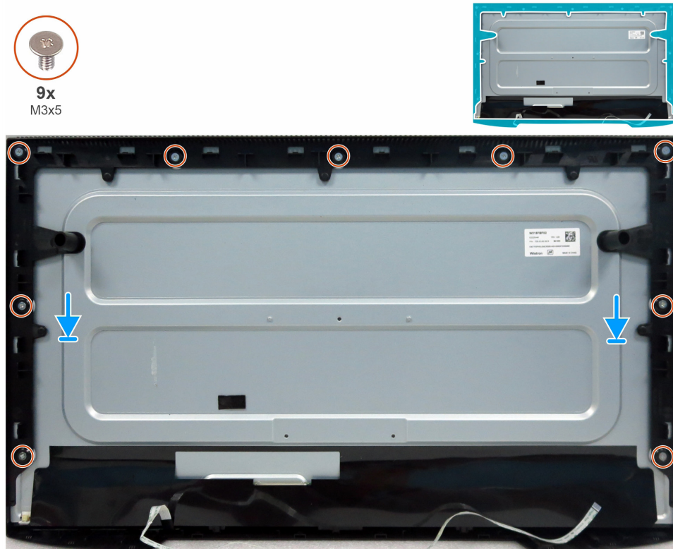
Figure 10. Installing the middle frame
