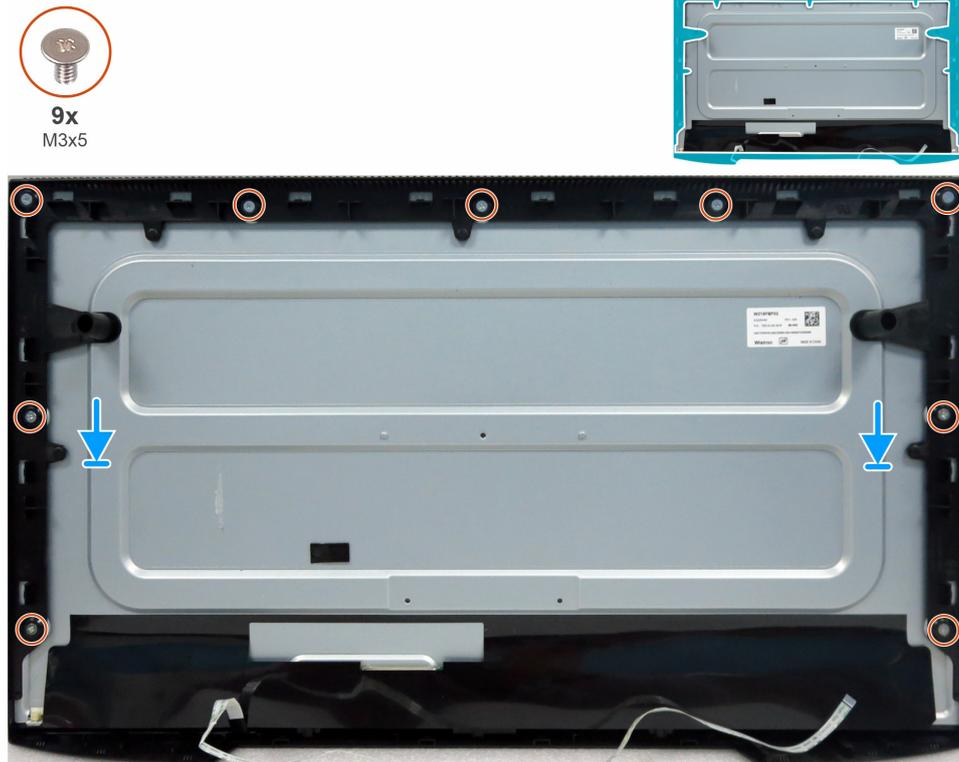
**Figure 19.** Installing the middle frame
