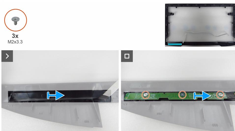
**Figure 20. Removing the keypad board**
