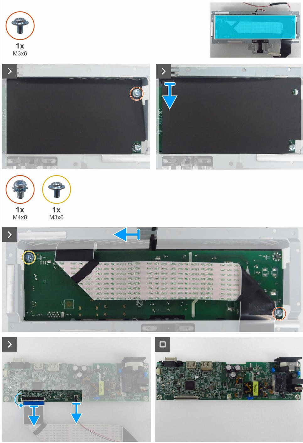
Figure 22. Removing the main board
