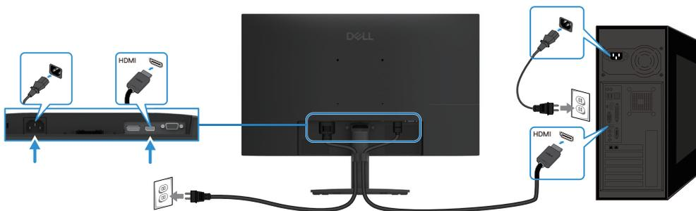
Figure 9. Connecting HDMI cable
