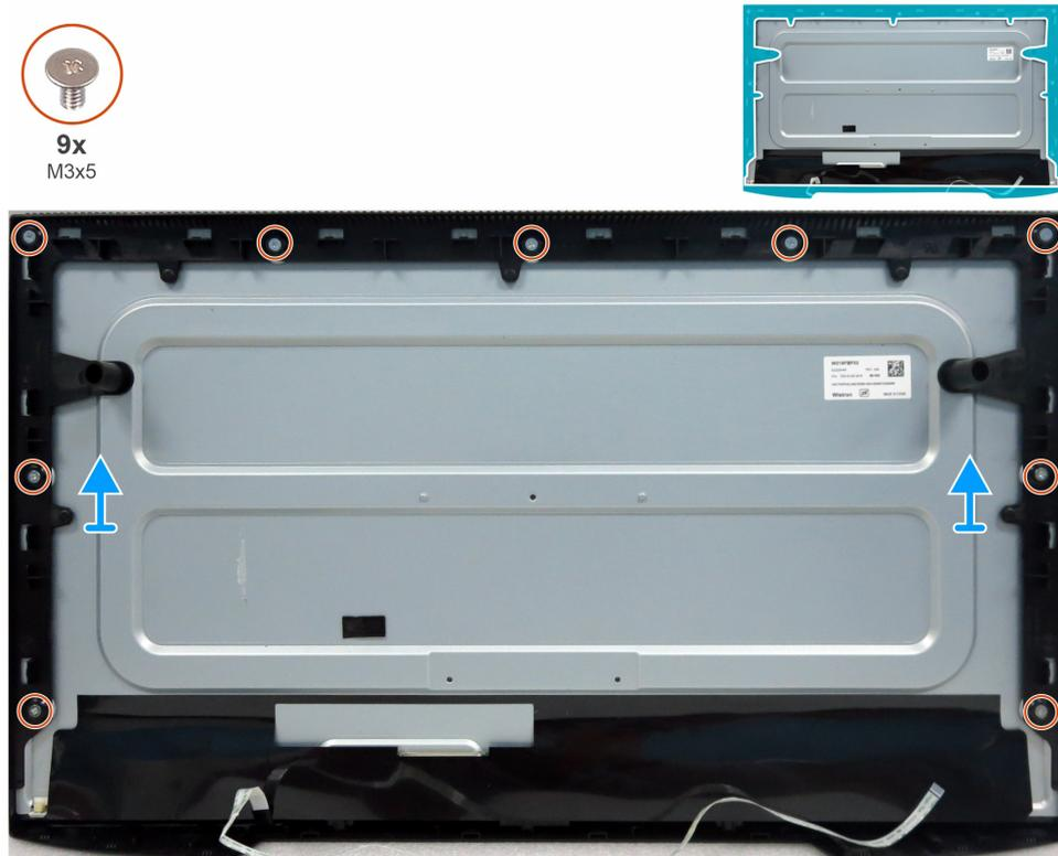
**Figure 18.** Removing the middle frame
