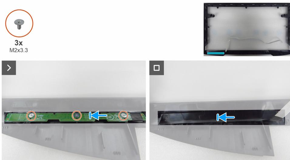
**Figure 21. Installing the keypad board**
