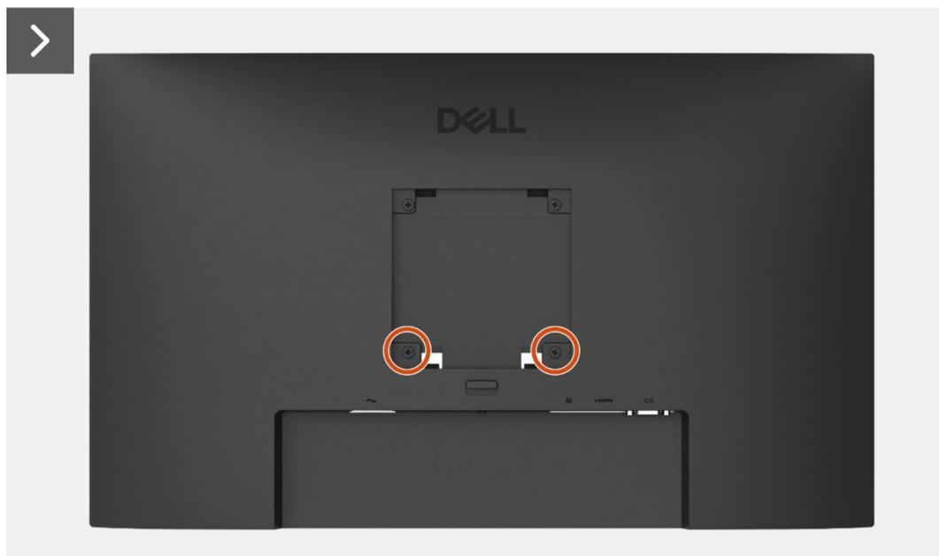
**Figure 3.** Removing the back cover
