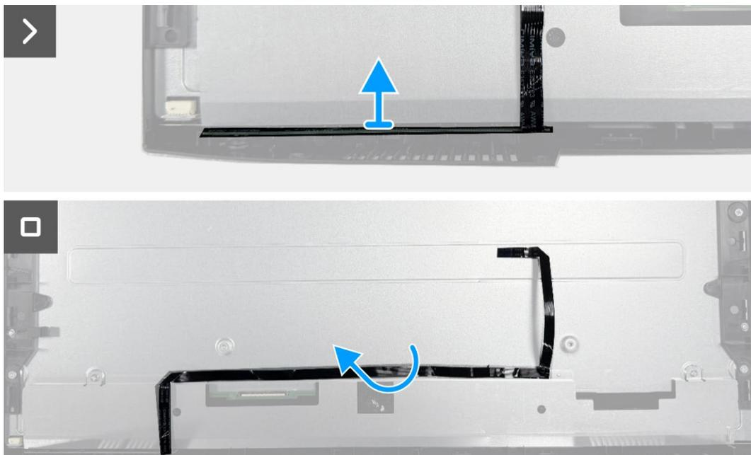
**Figure 13.** Removing the keypad board
