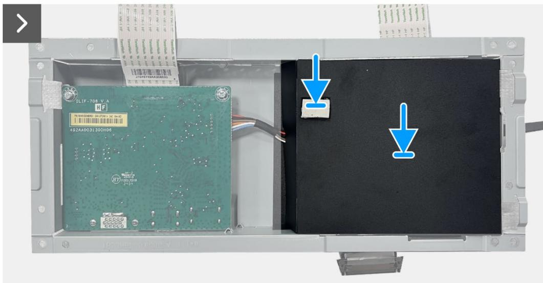
**Figure 41. Installing the interface board**
