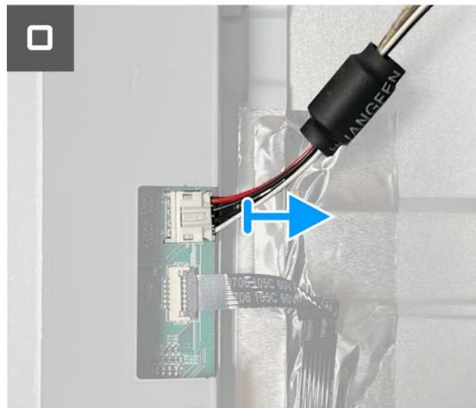
Figure 26. Removing the back cover
