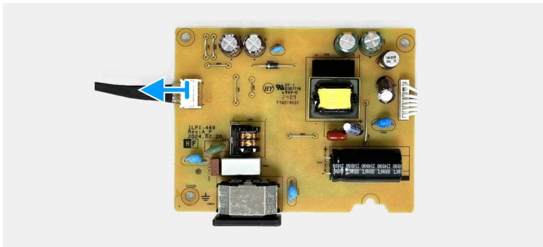
**Figure 43.** Removing the power board
