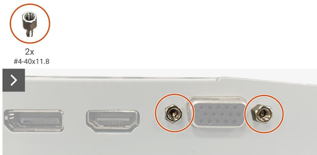
**Figure 37.** Removing the interface board
