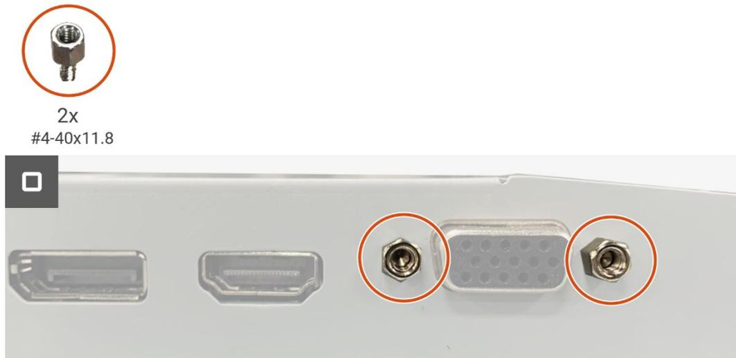
**Figure 42.** Installing the interface board
