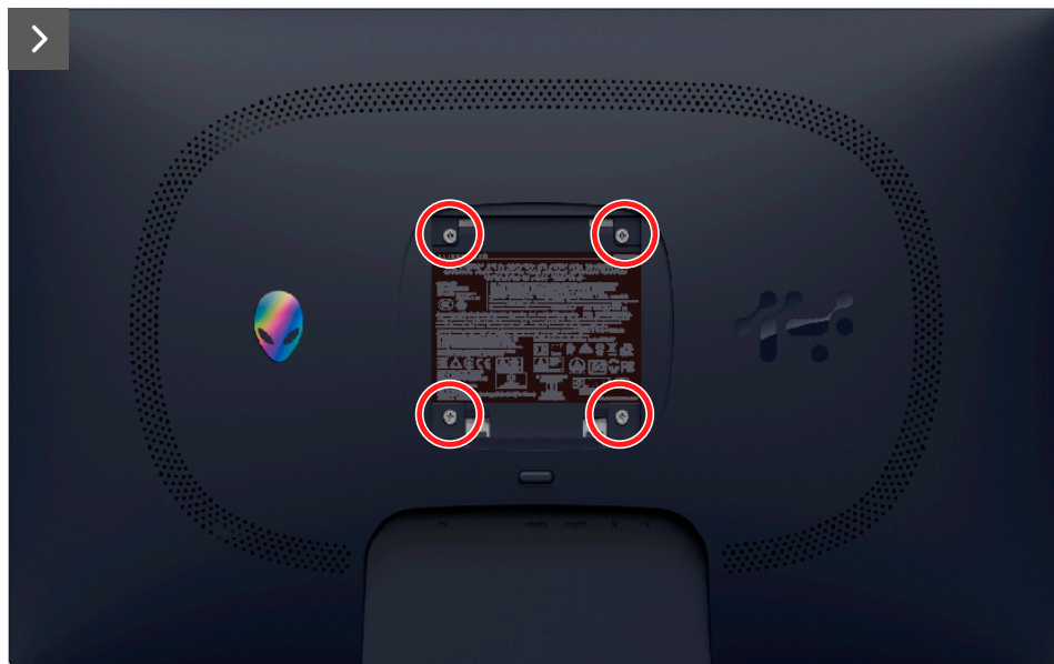
Figure 3. Removing the back cover
