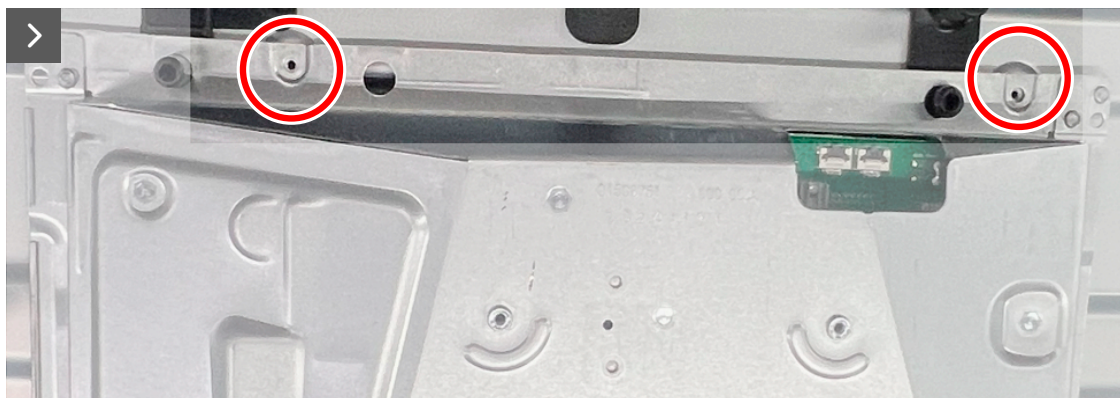
Figure 12. Removing the metal shield
