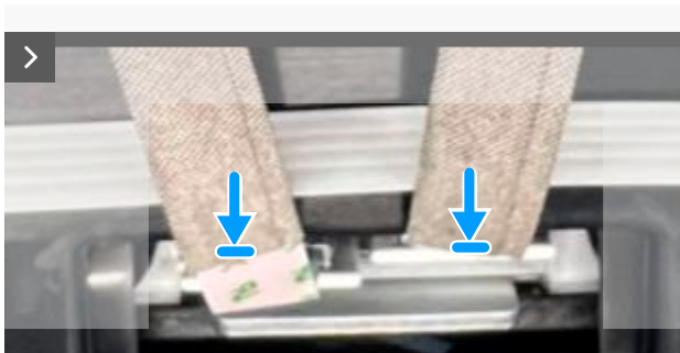
Figure 18. Installing the metal shield
