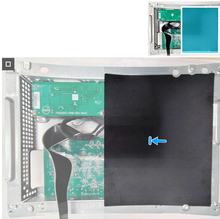
Figure 25. Installing the system board and power board
