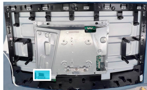
Figure 13. Removing the metal shield
