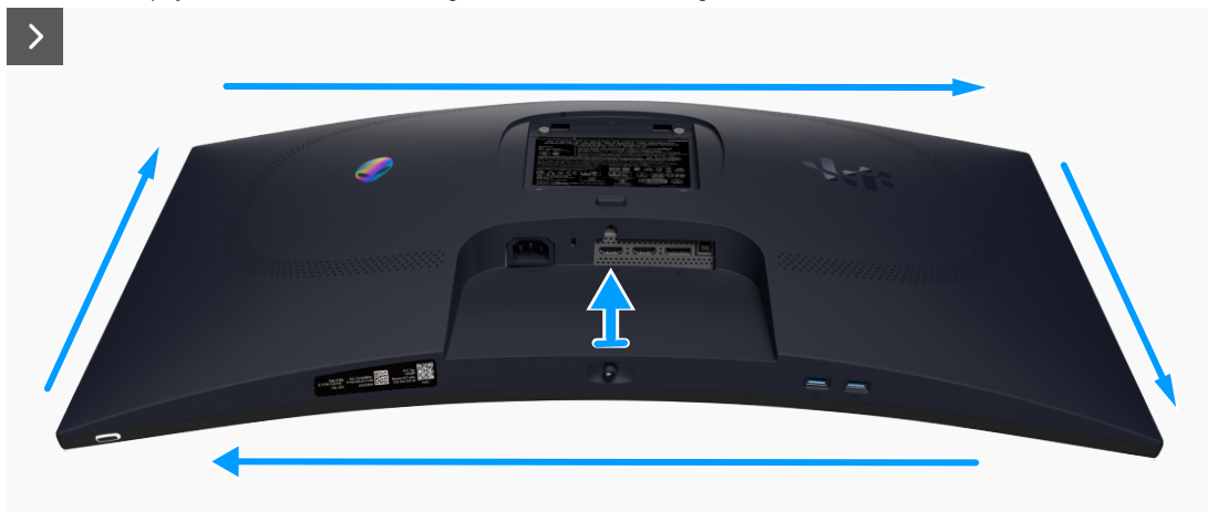
Figure 4. Removing the back cover
