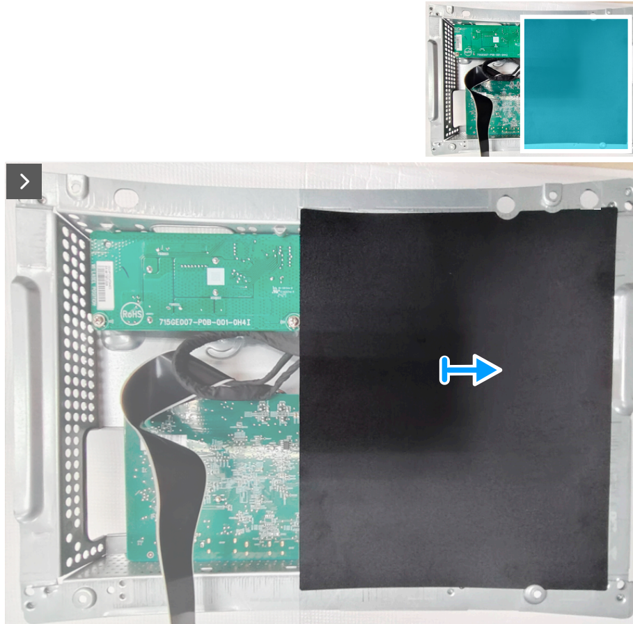
Figure 20. Removing the system board and power board
