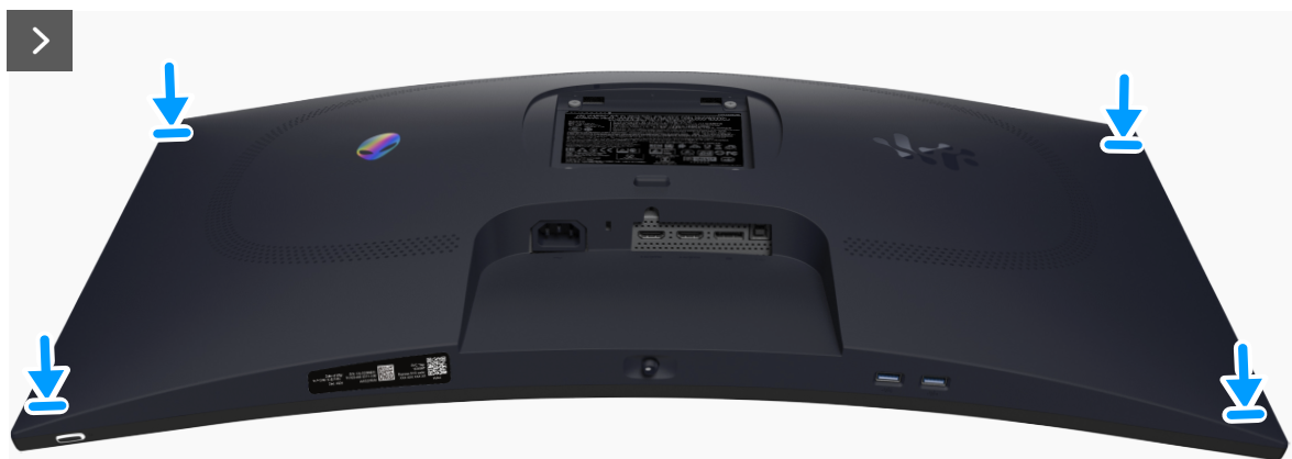
Figure 8. Installing the back cover
