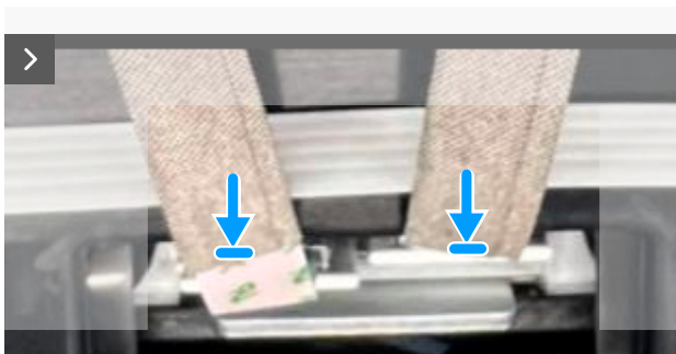
Figure 28. Installing the metal shield
