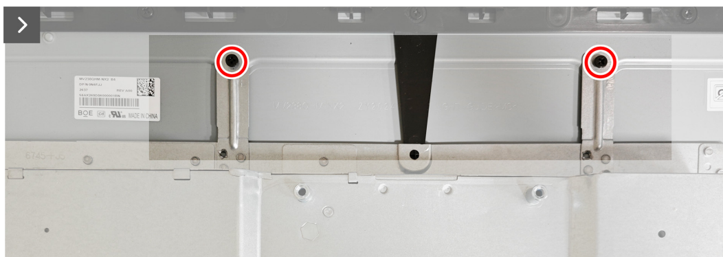
Figure 15. Installing the metal frame
