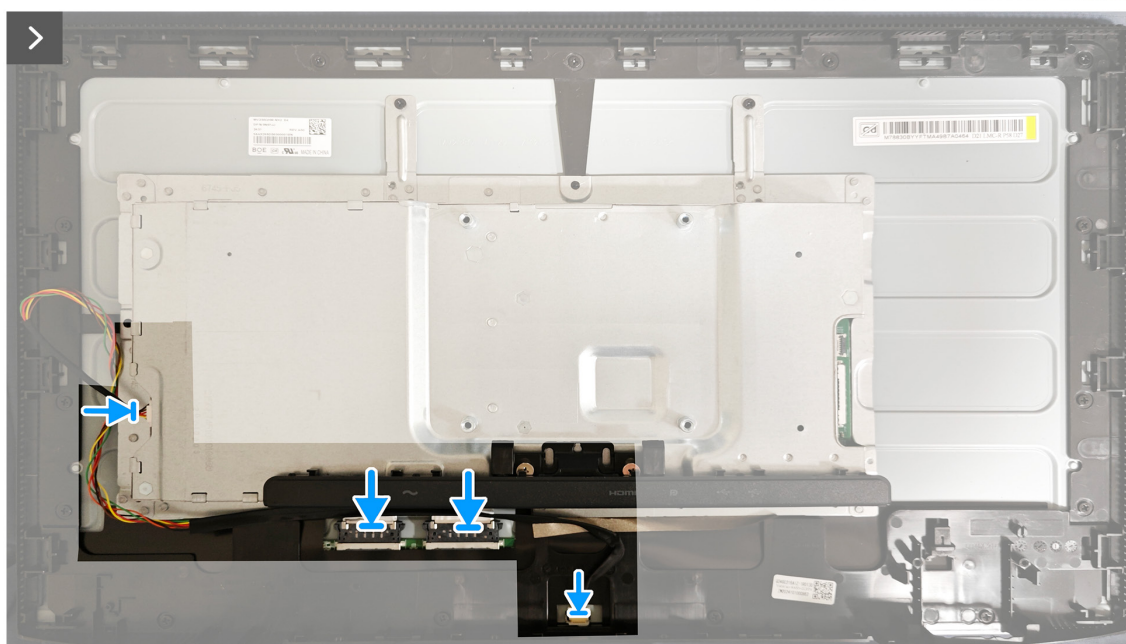
Figure 16. Installing the metal frame
