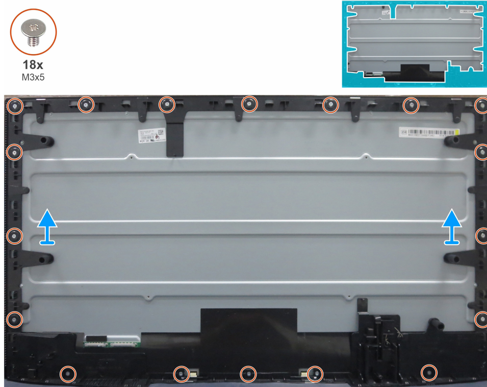
Figure 7. Removing the middle frame
