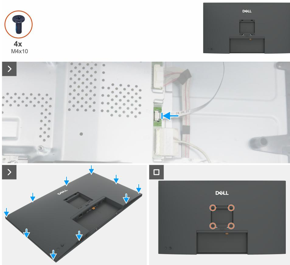
**Figure 18. Installing the back cover**
