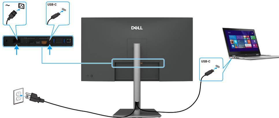
Figure 11. Connecting the USB-C to C cable
