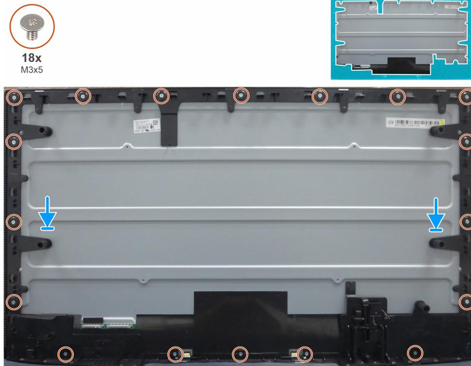
**Figure 28.** Installing the middle frame
