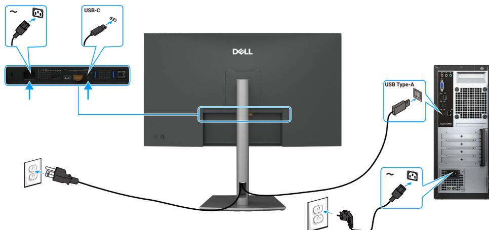
Figure 13. Connecting the USB Type-C to Type-A cable
