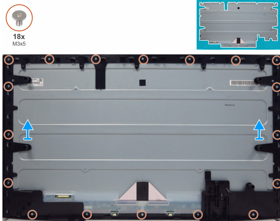
Figure 7. Removing the middle frame
