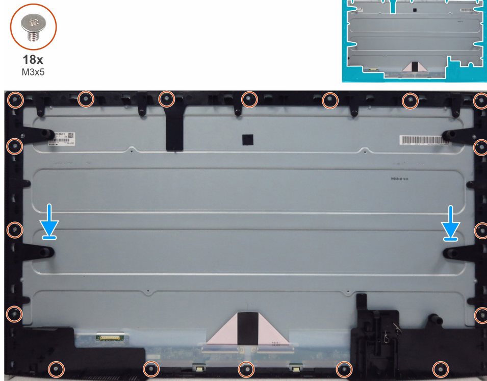
Figure 26. Installing the middle frame
