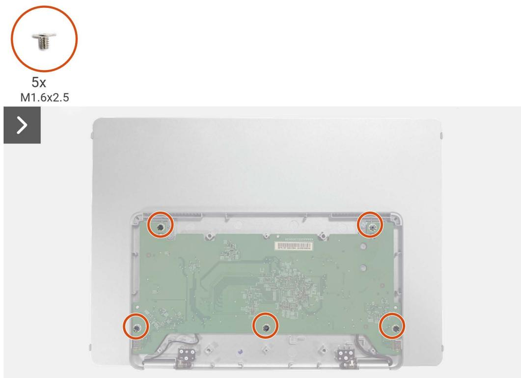
**Figure 15.** Removing the main board
