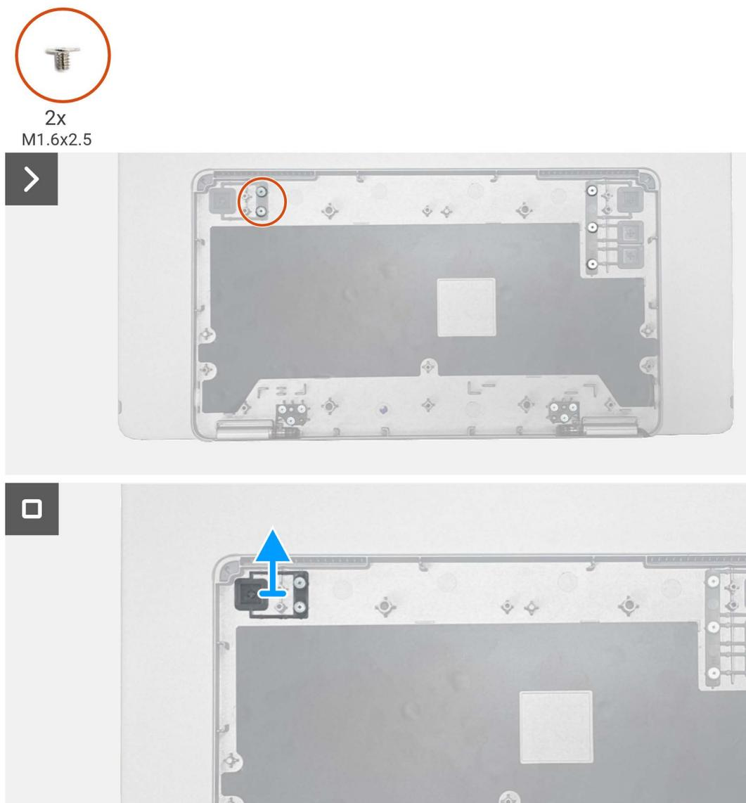
**Figure 28.** Removing the power button
