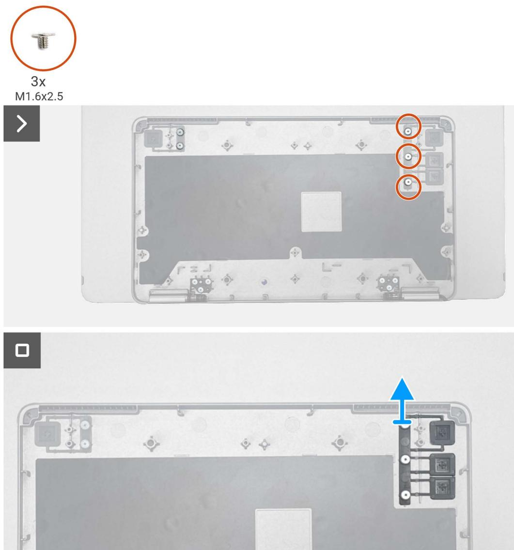
**Figure 30.** Removing the function button
