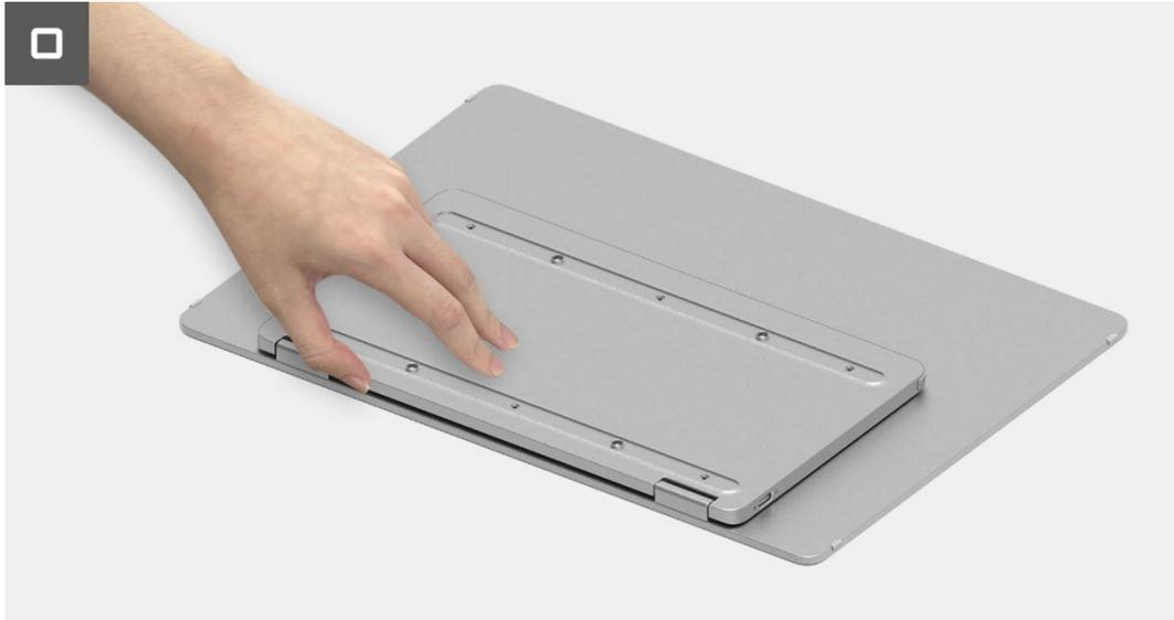
**Figure 13.** Removing the bottom base cover
