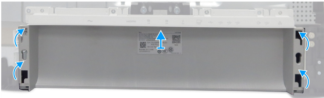
Figure 4. Removing the lower back cover
