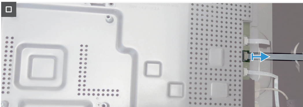
Figure 2. Removing the upper back cover
