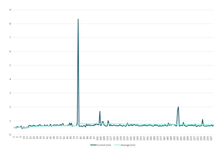
FIGURE 3. Current and average time to service I/O requests with indexing rate of 2 TB per day and simultaneous heavy search load
