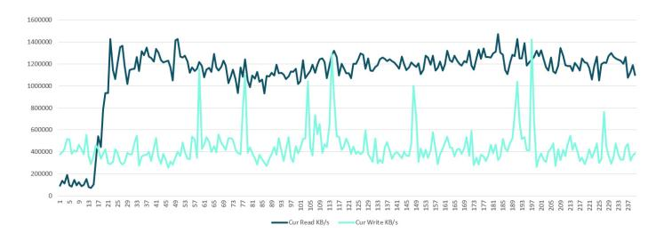
FIGURE 4. Array throughput with HPE Primera all-flash array at an indexing rate of 2 TB per day and simultaneous heavy search load
