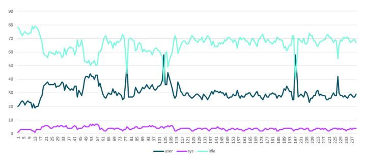
FIGURE 6. CPU utilization of HPE Primera all-flash array at an indexing rate of 2 TB per day and simultaneous heavy search load
