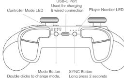
Double clicks to change mode. Long press for power off, short press for power on. Long press 2 seconds above to start scrolling
