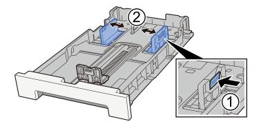
2 Adjust the paper length guide to the paper size required. Press the paper length adjusting tab and slide the guides to the paper size required.
