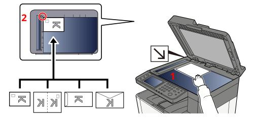
2 Align it flat against the original size indicator plates with the back left corner as the reference point.
