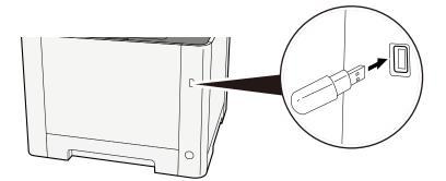
When the machine recognizes the USB drive, the message "USB Drive is recognized. Displaying files." appears.
