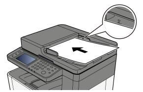
Ensure that loaded originals do not exceed the level indicator. Exceeding the maximum level may cause the originals to jam.
