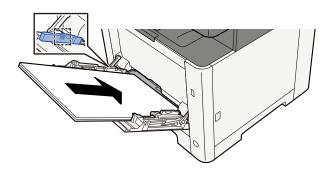
Insert the paper along the paper width guides into the tray until it stops.
