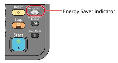
If print data is received during Sleep, the machine automatically wakes up and starts printing.
