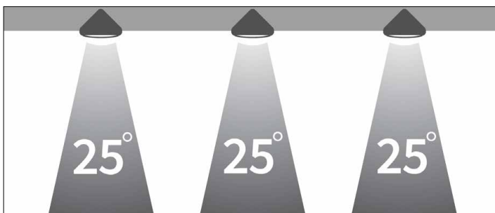
LIMITED DISPERSION: A typical in-ceiling speaker's tight dispersion pattern creates a very limited listening area and requires a larger number of speakers to give adequate coverage in the living space.
