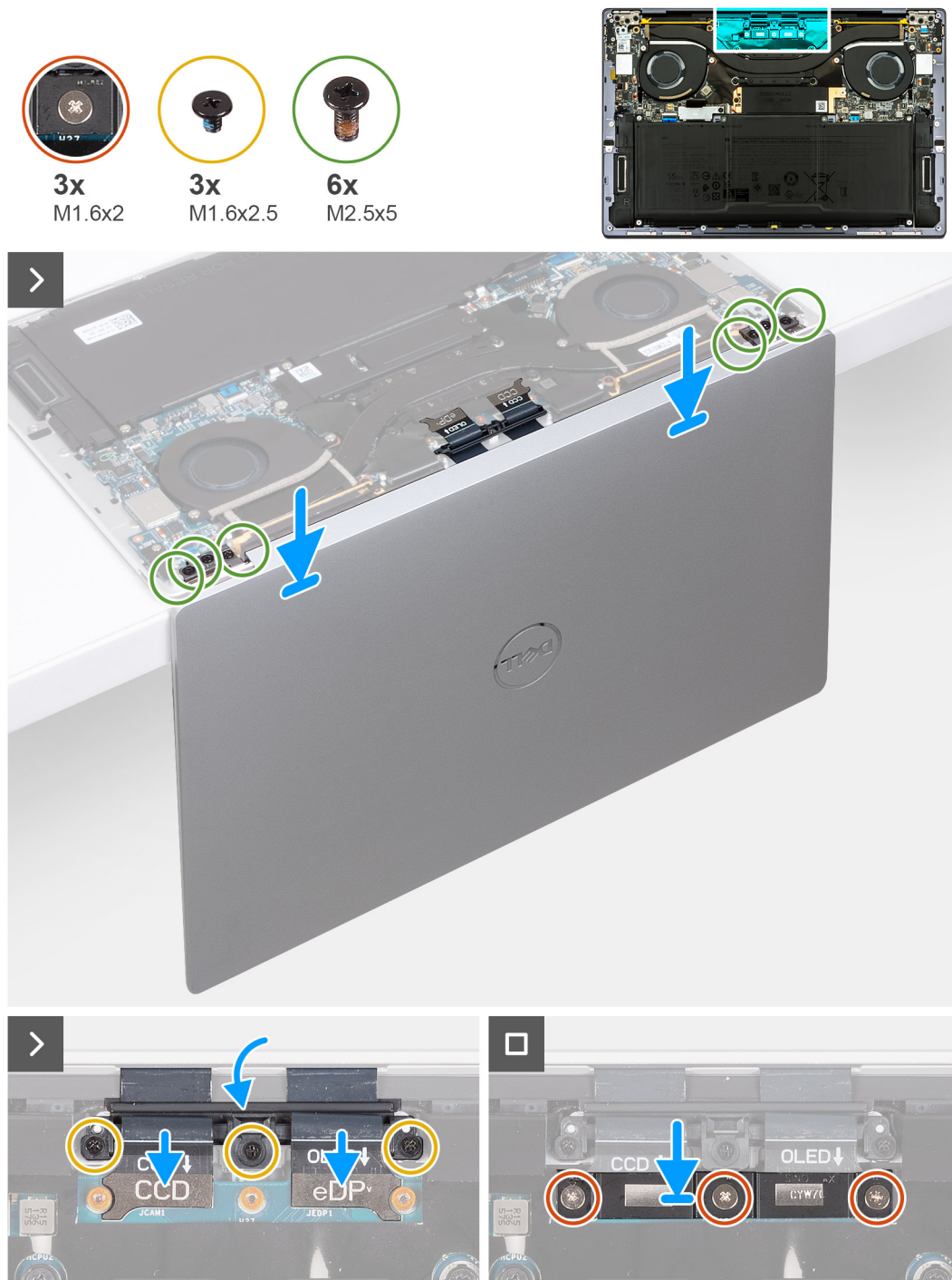
Figure 33. Installing the display assembly
