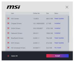
Check the Select All checkbox in the lower-left corner and click Install to install MSI Center and drivers. The installation progress will be shown at the bottom.
