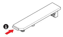
2. Slightly lift up the end part of Screwless M.2 Shield Frozr heatsink and move it forward to uninstall the heatsink.
