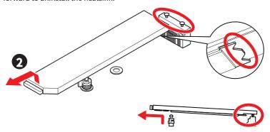
If you install 2260 SSD, use the included EZ M.2 Clip II Remover. Place the included EZ M.2 Clip II in the slot, use the remover to screw it in by turning clockwise, and secure it. Skip this step if you install 2280 SSD.
