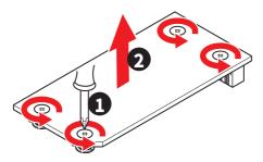
3. If you install 2260 SSD, use the included EZ M.2 Clip II Remover. Place the included EZ M.2 Clip II in the slot, use the remover to screw it in by turning clockwise, and secure it. Skip this step if you install 2280 SSD.
