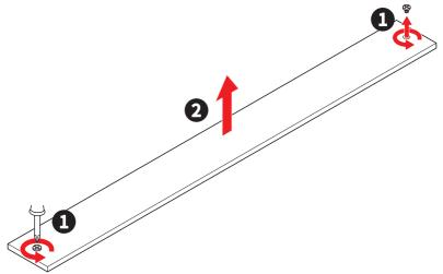
If you want to install the 2260 SSD in M2\_3 slot or the 22110 SSD in M2\_2 slot, replace the EZ M.2 Clip II to the 2260 or 22110 hole. Please note that you have to use the EZ M.2 Chip II Remover to remove and install the EZ M.2 Clip II. Skip this step if you install 2280 SSD.
