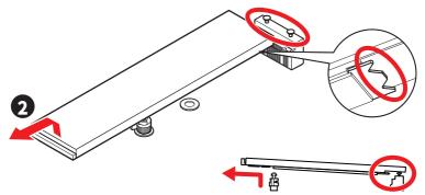
3. If you install 2260 SSD, use the included **EZ M.2 Clip II Remover**. Place the included **EZ M.2 Clip II** in the slot, use the remover to screw it in by turning clockwise, and secure it. Skip this step if you install 2280 SSD.
