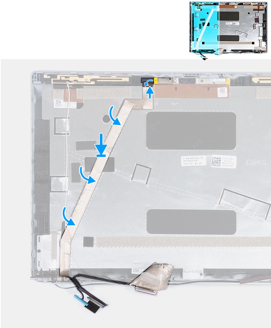
**Figure 52. Installing the display cable**
