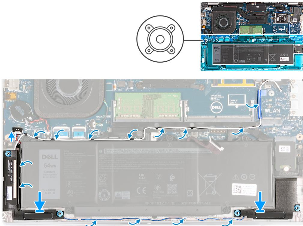
**Figure 32. Installing the speakers**
