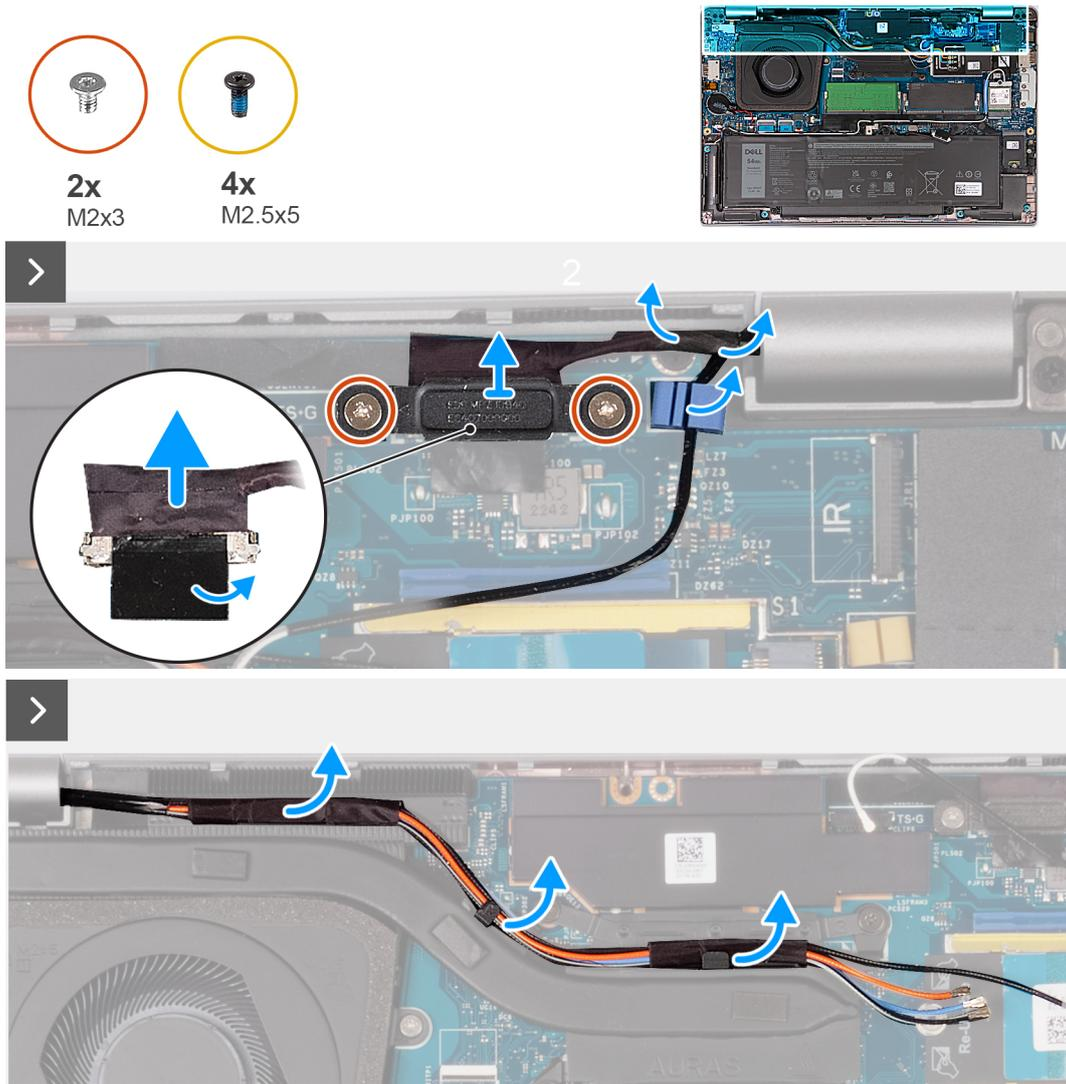
Figure 37. Removing the display assembly - For computers shipped with 5G card
