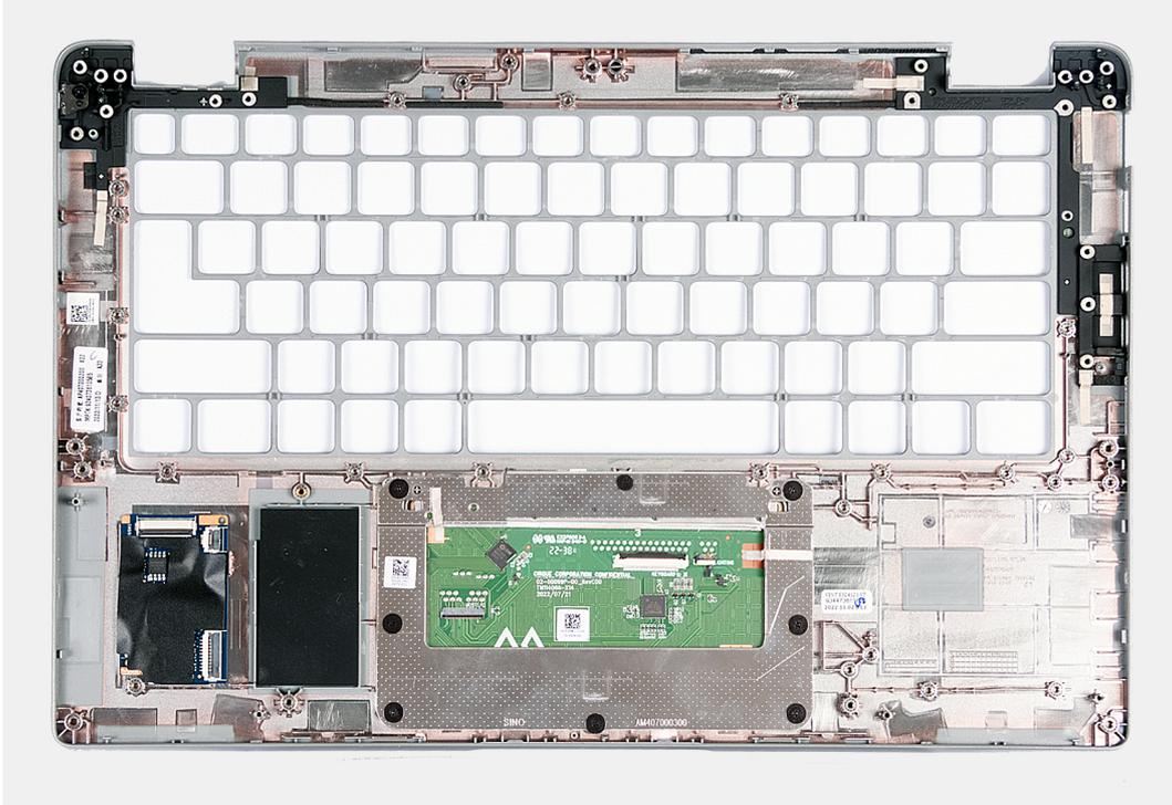
**Figure 67. Removing the palm-rest assembly**
