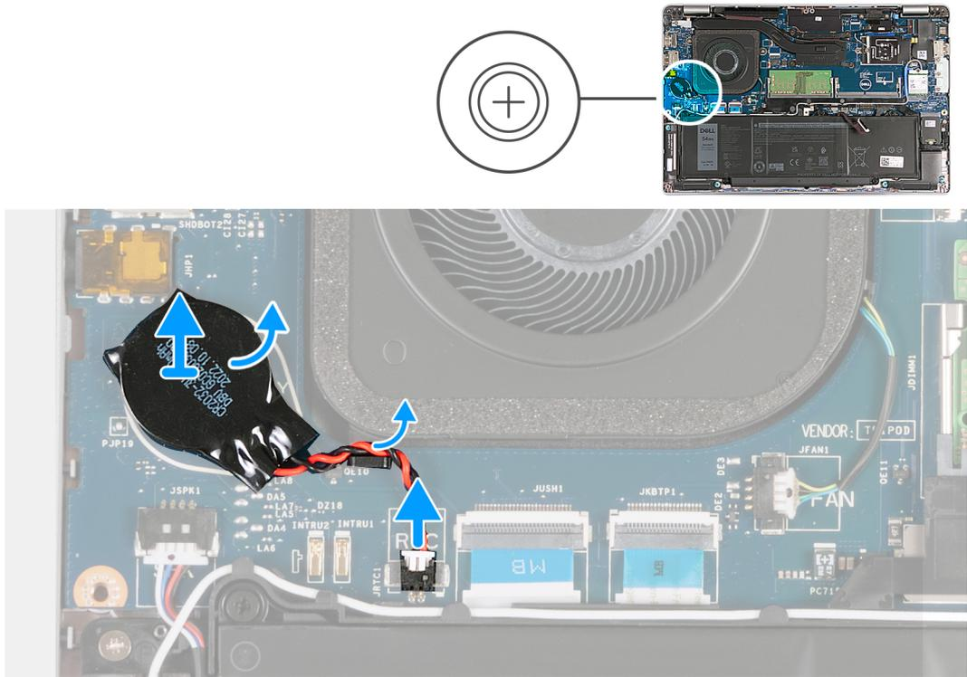
**Figure 22. Removing the coin-cell battery**
