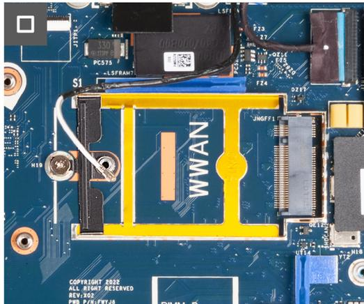
Figure 14. Removing the WWAN card - For computers shipped with 4G card
