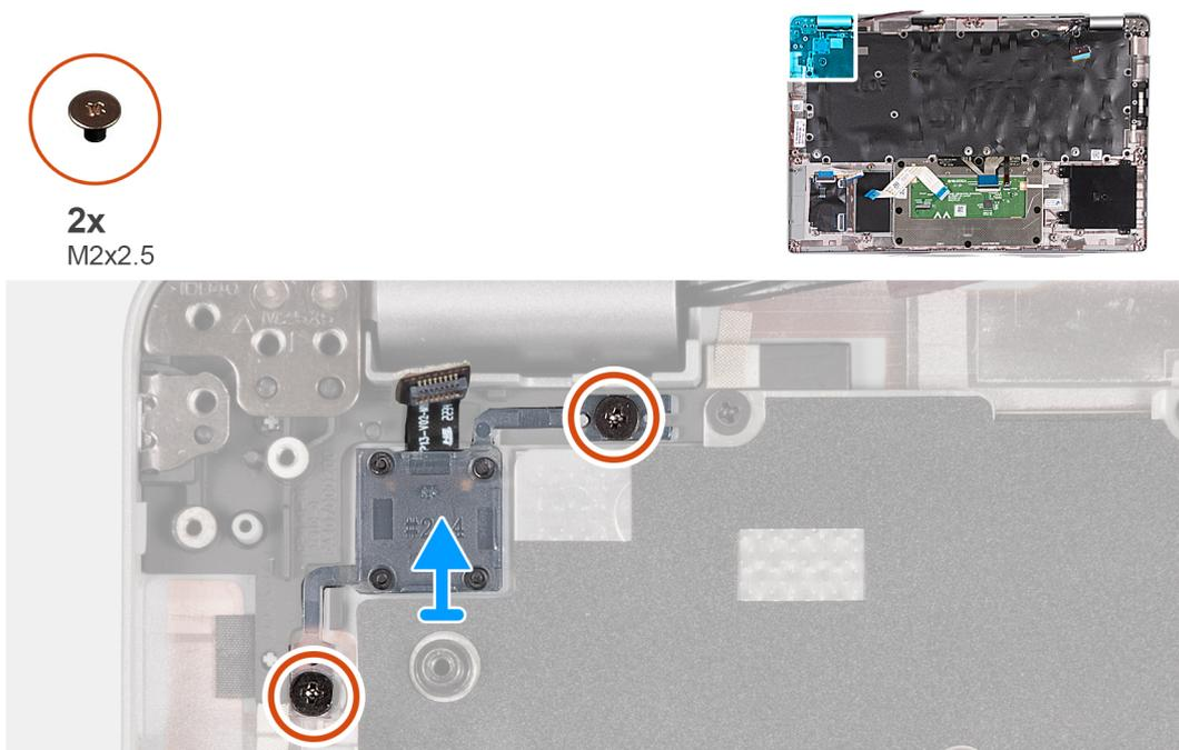
**Figure 63. Removing the power-button board**
