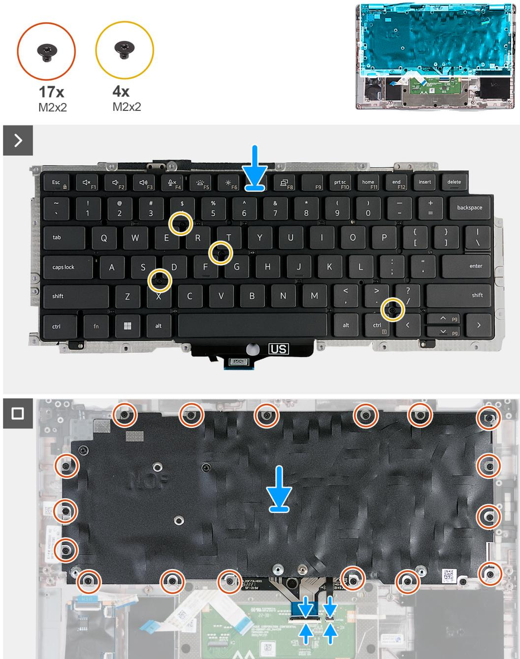
Figure 66. Installing the keyboard
