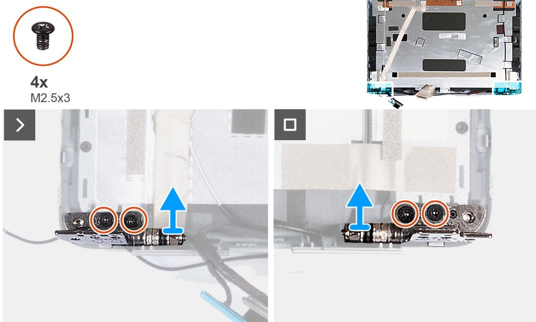
**Figure 49. Removing the display hinges**
