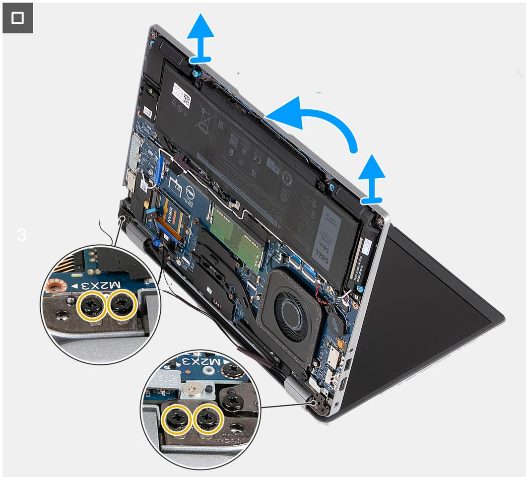
**Figure 38. Removing the display assembly - For computers shipped with 5G card**
