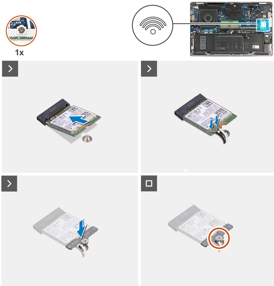
**Figure 13. Installing the wireless card**
