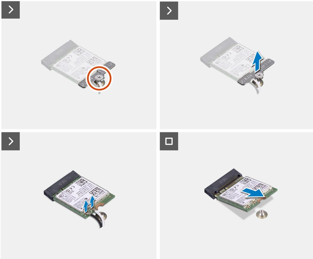
**Figure 12. Removing the wireless card**
