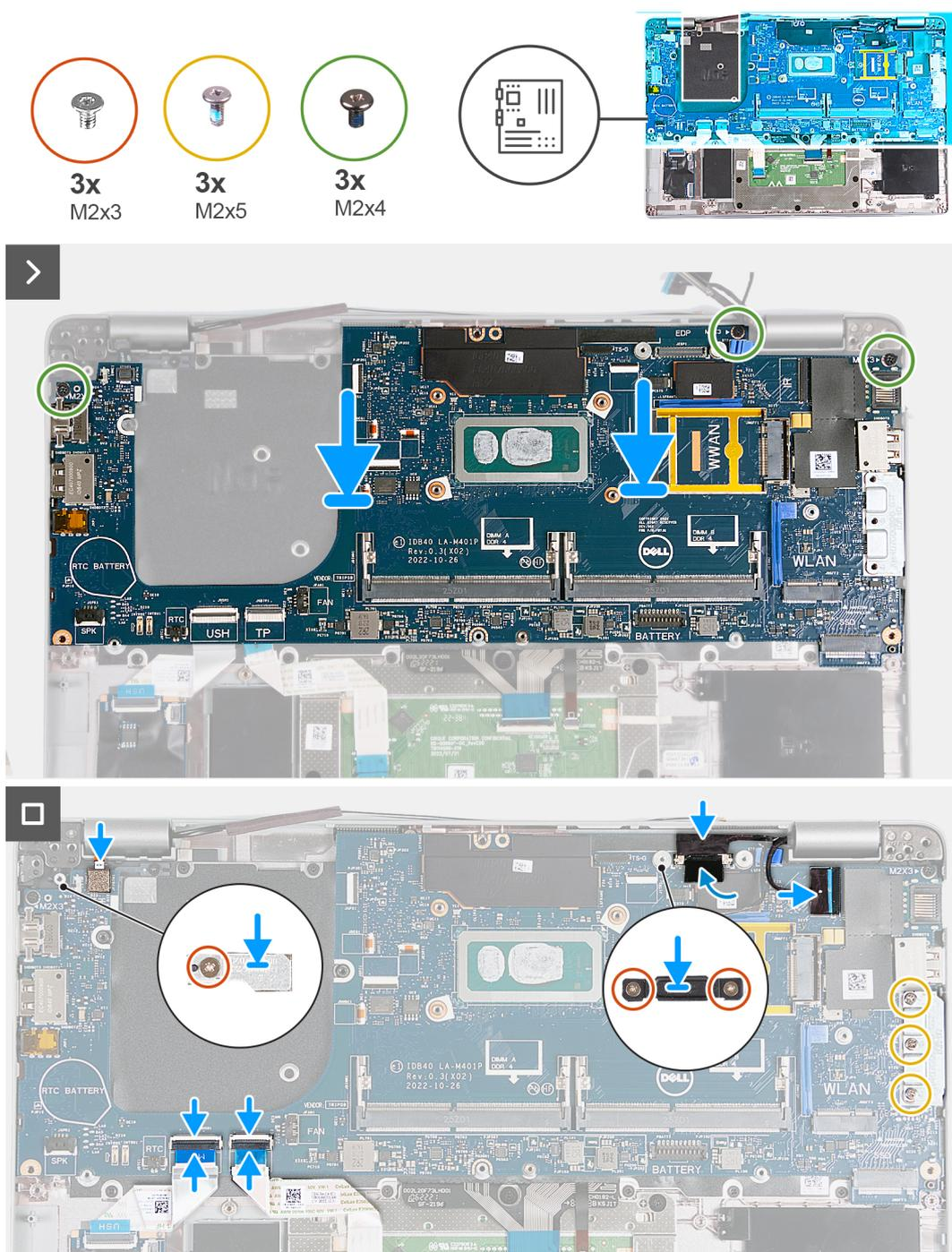
**Figure 60. Installing the system board**
