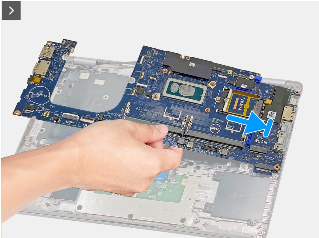
Figure 59. Installing the system board
