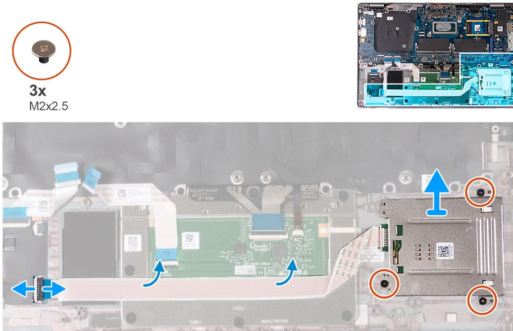
Figure 61. Removing the smart card reader
