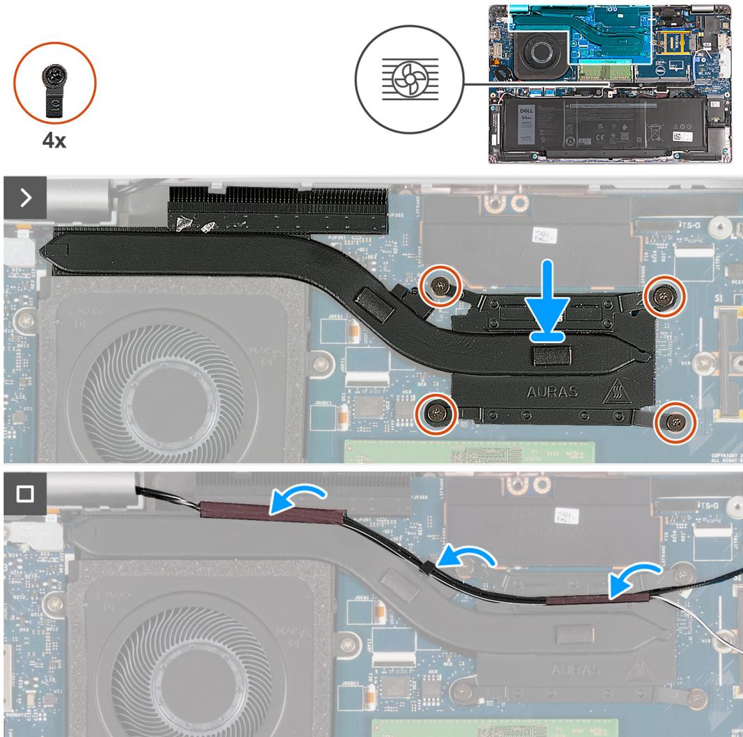
Figure 27. Installing the heat sink - For computers shipped with 4G card
