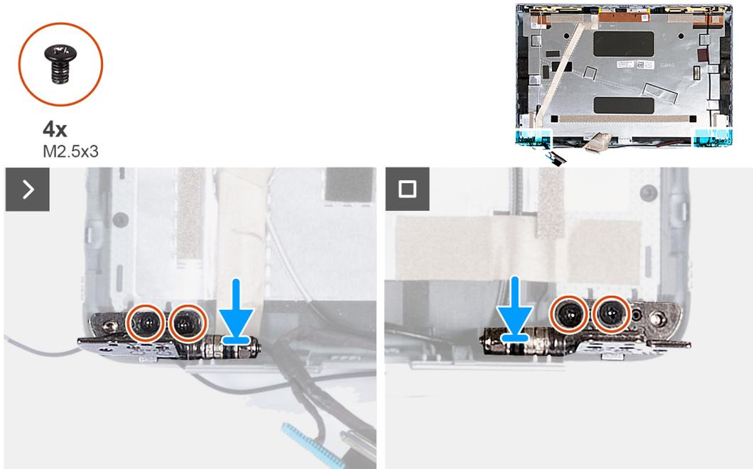
**Figure 50. Installing the display hinges**
