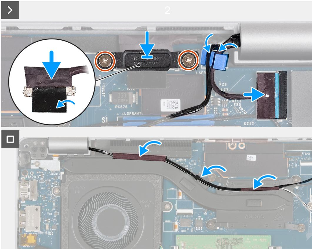
Figure 40. Installing the display assembly - For computers shipped with 4G card
