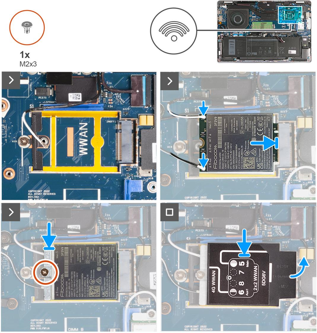
Figure 16. Installing the WWAN card - For computers shipped with 4G card
