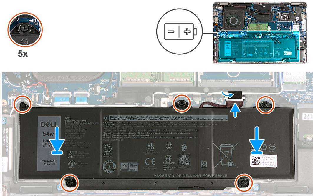
**Figure 21. Installing the battery**
