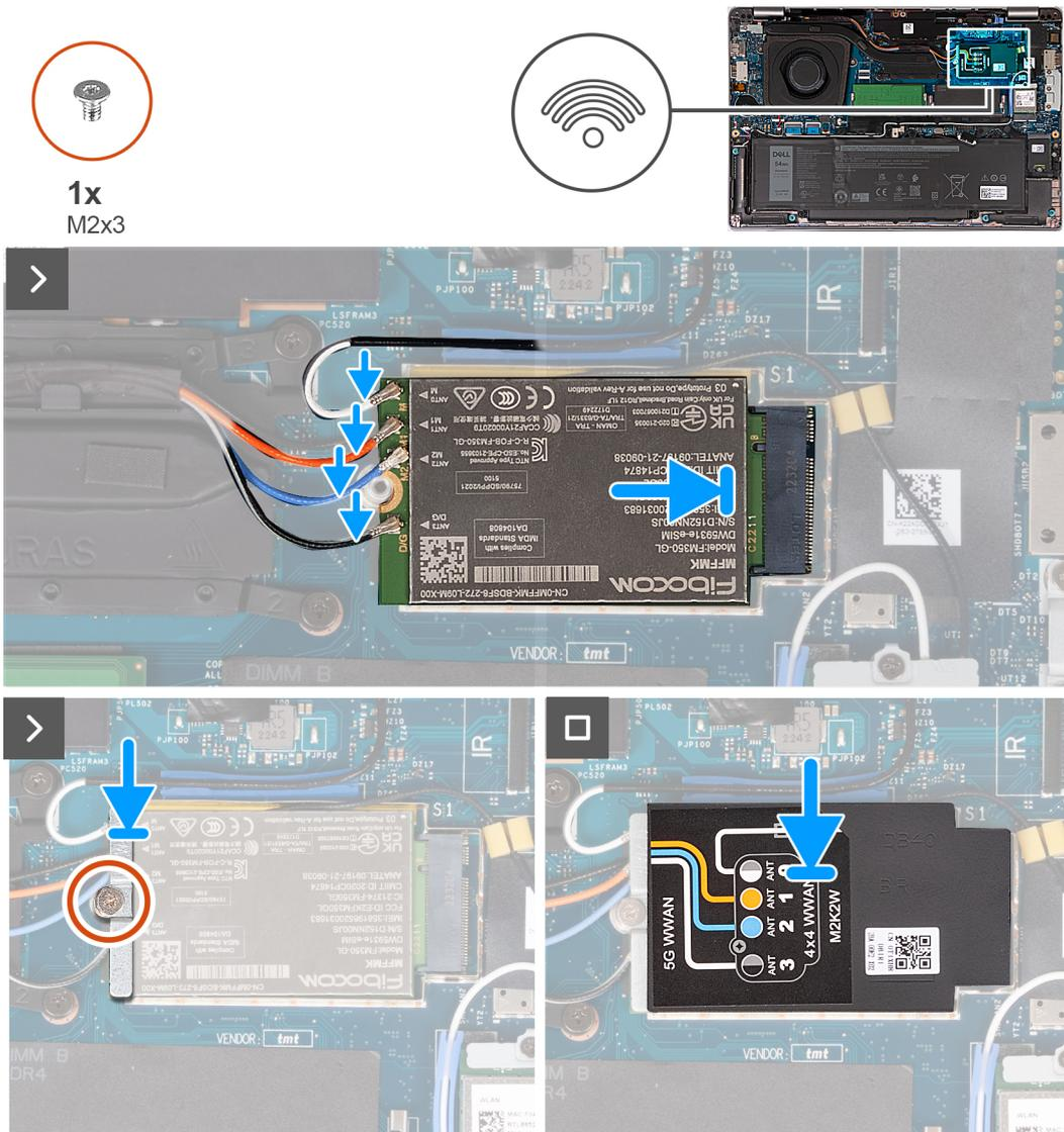
Figure 17. Installing the WWAN card - For computers shipped with 5G card
