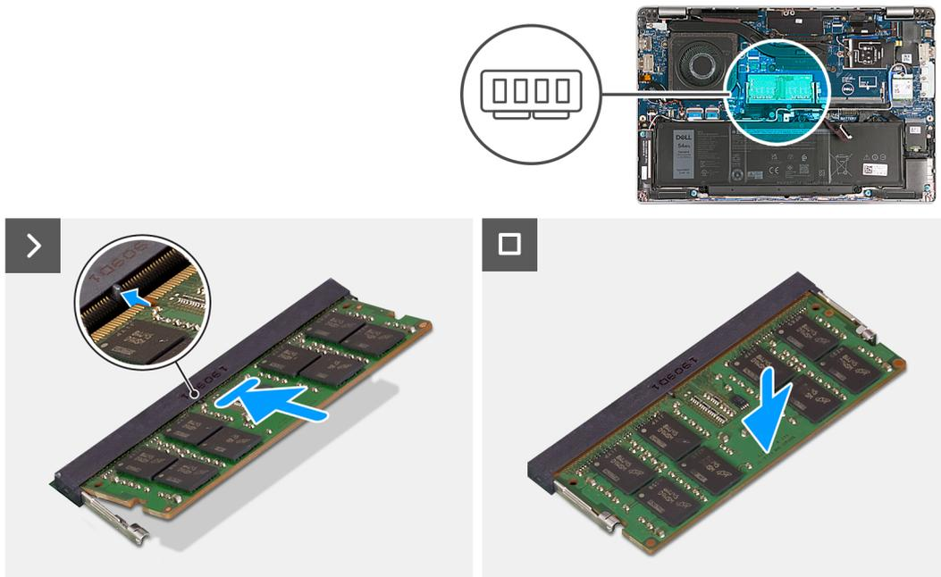
Figure 9. Installing the memory module
