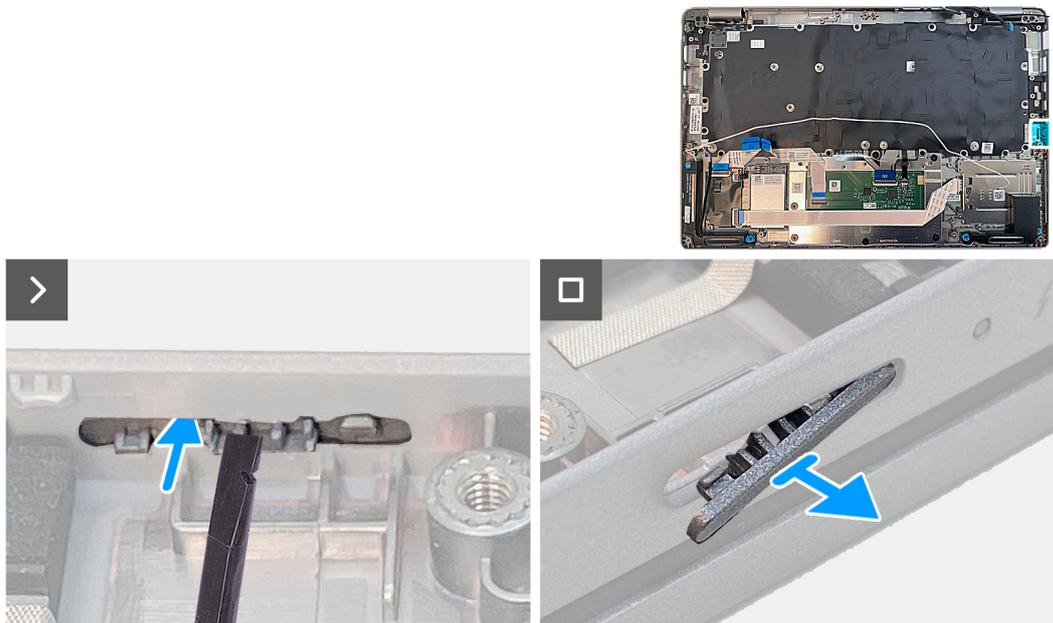
Figure 69. Removing the dummy SIM-card slot filler
