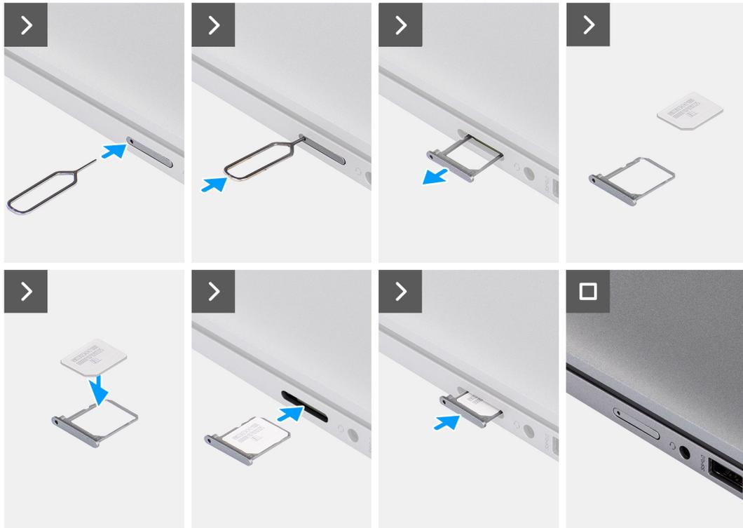
Figure 5. Installing the nanoSIM card
