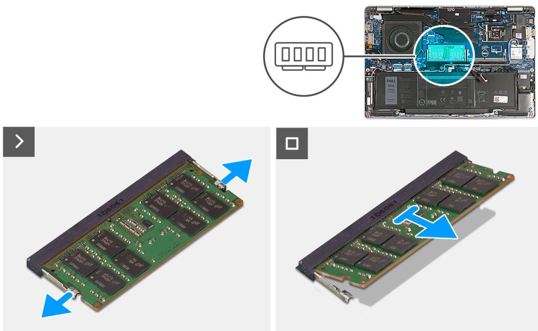
**Figure 8. Removing the memory module**
