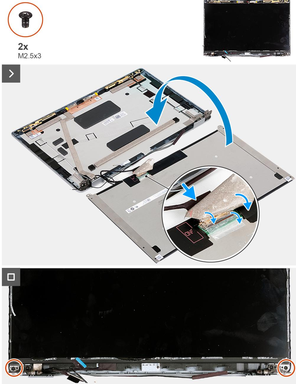
**Figure 46. Installing the display panel**
