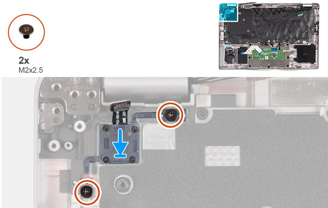
**Figure 64. Installing the power-button board**
