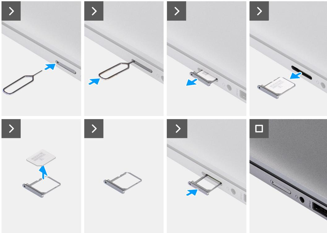
**Figure 4. Removing the nanoSIM card**
