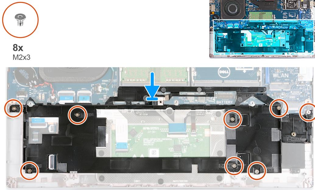
**Figure 34. Installing the assembly inner frame**
