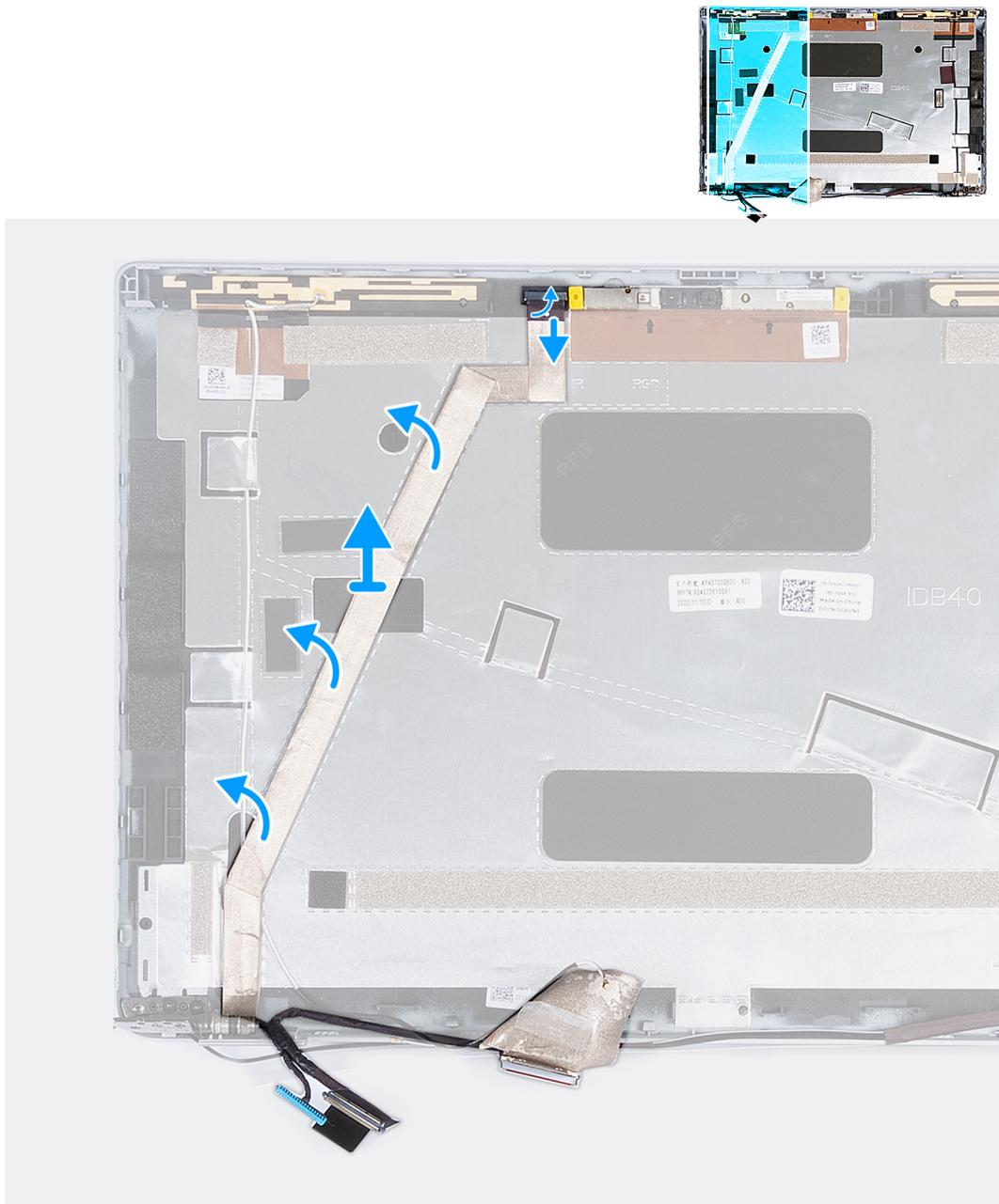
**Figure 51. Removing the display cable**
