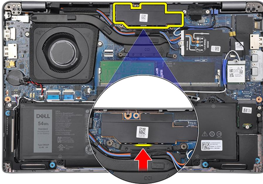
Figure 26. Power shielding cover
