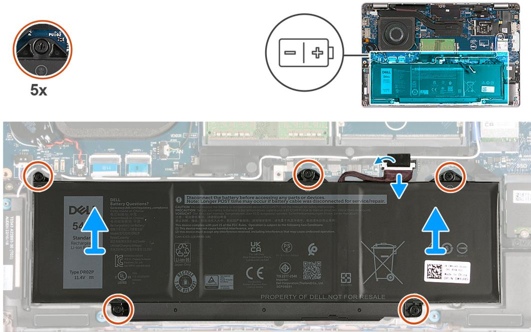
Figure 20. Removing the battery
