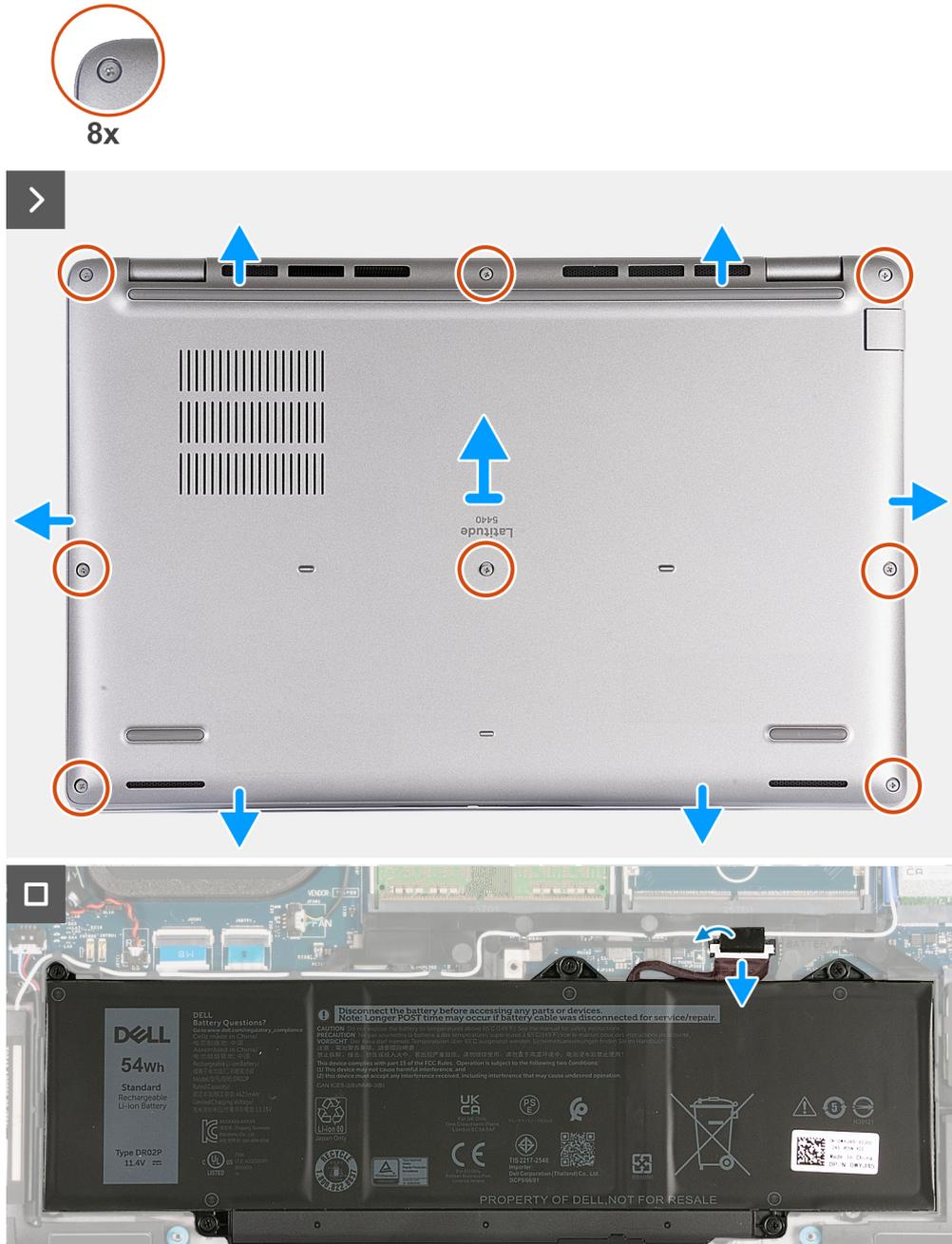
**Figure 6. Removing the base cover**
