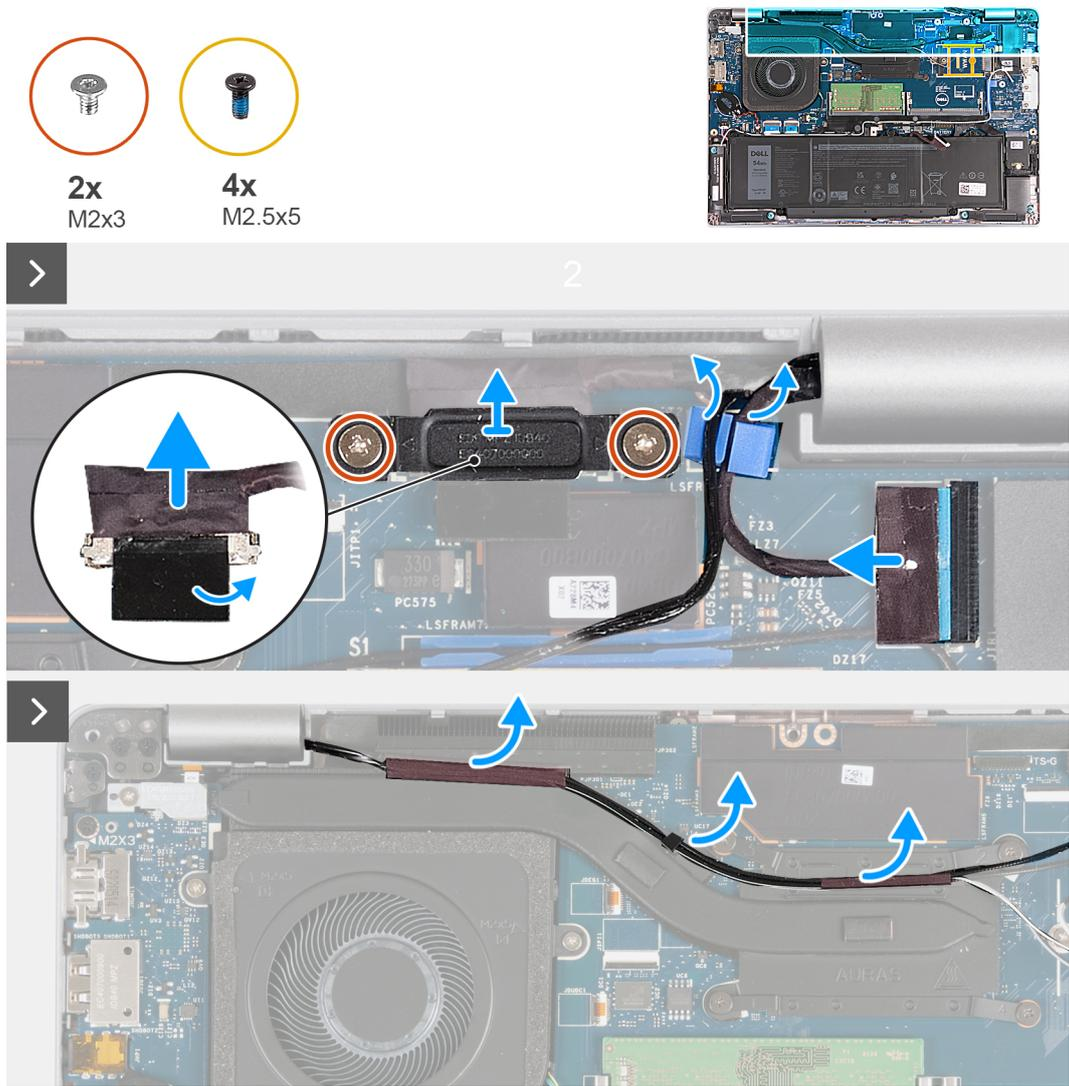
**Figure 35. Removing the display assembly - For computers shipped with 4G card**
