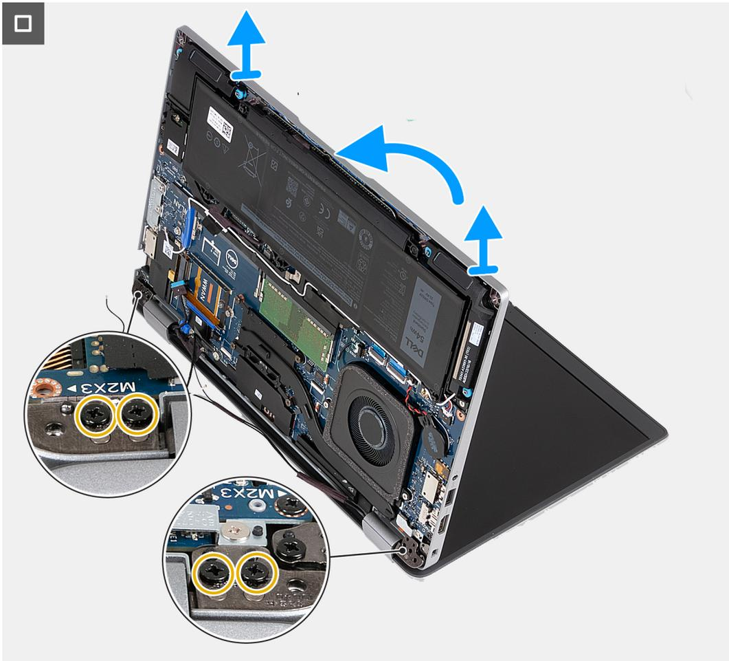
Figure 36. Removing the display assembly - For computers shipped with 4G card
