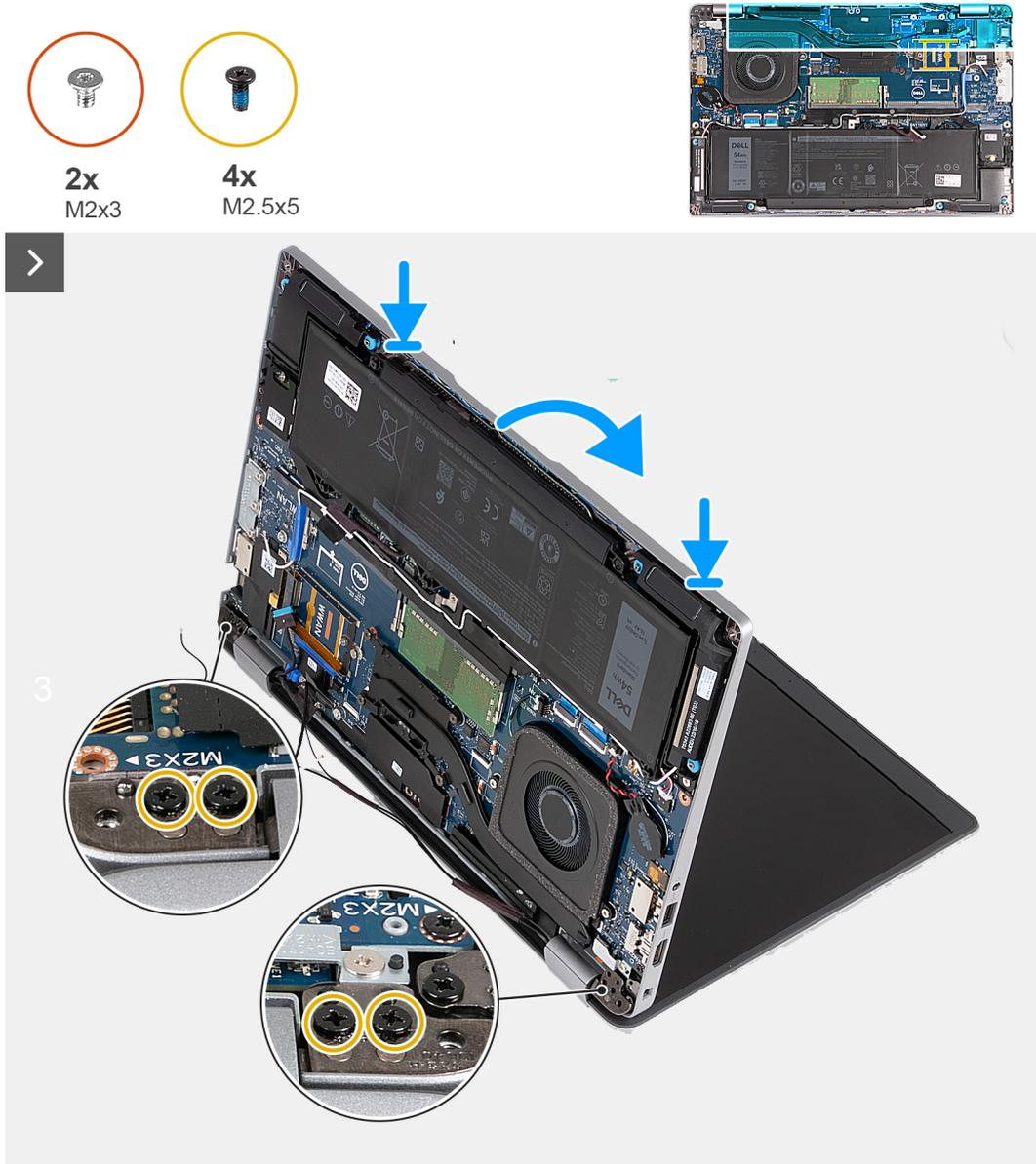
Figure 39. Installing the display assembly - For computers shipped with 4G card
