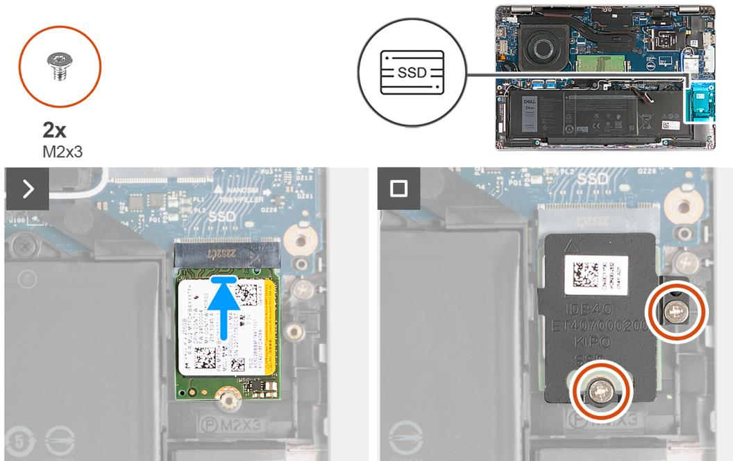
**Figure 11. Installing the M.2 2230 solid-state drive**
