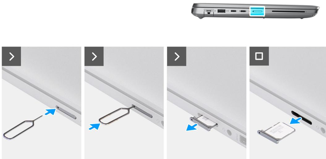
Figure 2. Removing the SIM card tray
