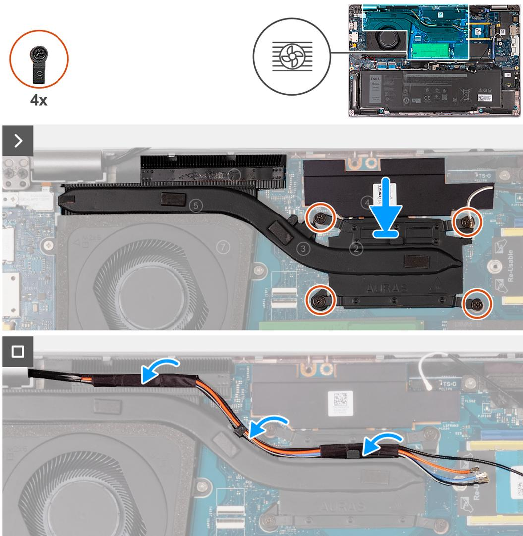
**Figure 28. Installing the heat sink - For computers shipped with 5G card**
