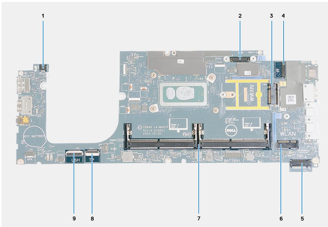
**Figure 58. System board connectors**
