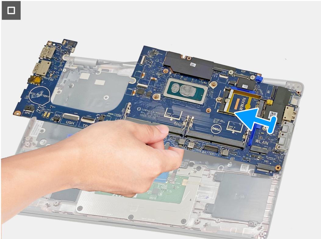
**Figure 57. Removing the system board**
