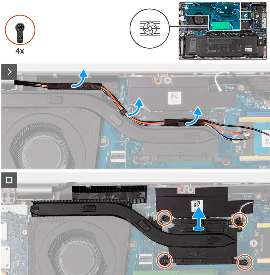
**Figure 25. Removing the heat sink - For computers shipped with 5G card**
