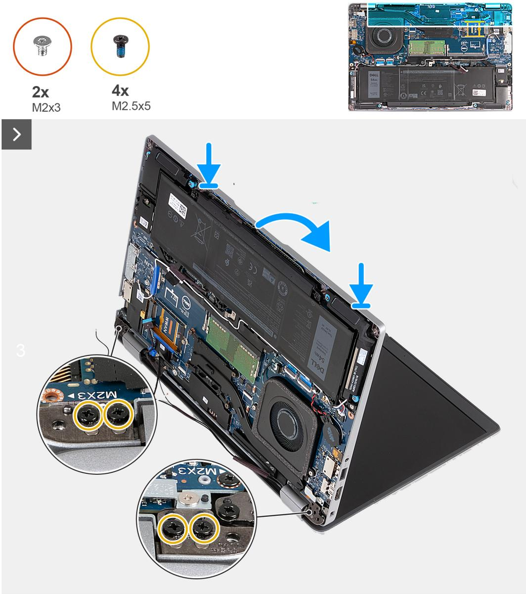
Figure 41. Installing the display assembly - For computers shipped with 5G card
