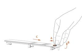
Push and hold the button on the M.2 heatsink (A). Then lift up the heatsink (B) and move it in the direction shown (C).
