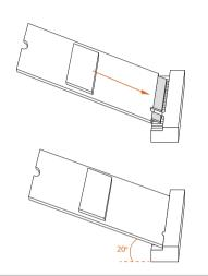
Align and gently insert the M.2 SSD into the M.2 slot. Please be aware that the M.2 SSD only fits in one orientation.
