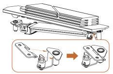
Hook the tab of the M.2 heatsink back onto the standoff.
