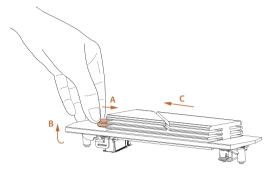
Push the button on the M.2 heatsink in the direction shown (A). Then lift up the heatsink (B) and move it in the direction shown (C).
