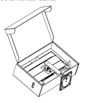
2. While keeping the release button pressed, tilt the base and slide it out.
