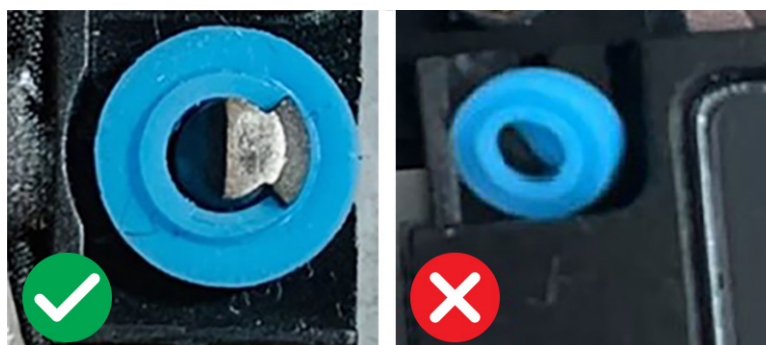
Figure 40. Seating position of the rubber grommets
