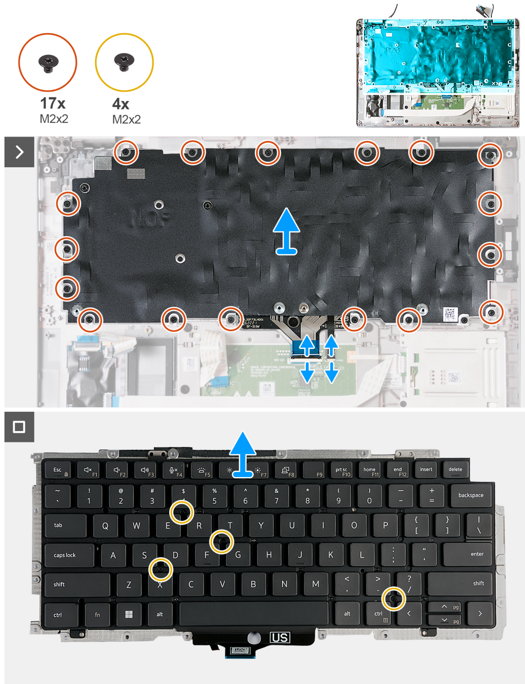
Figure 79. Removing the keyboard
