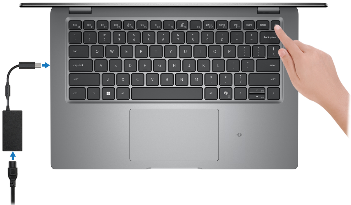
Figure 1. Connect power adapter and press the power button
