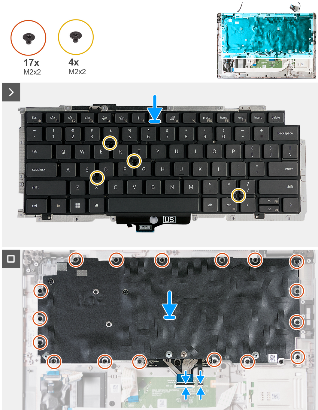
Figure 81. Installing the keyboard
