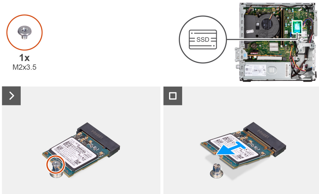
Figure 17. Removing the M.2 2230 solid-state drive
