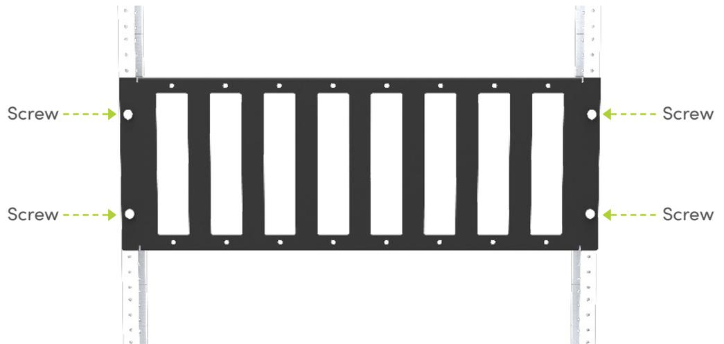
2. Install the ZyPer4K encoders/decoder in the carrier unit using the included 4-40 countersink screws. ZyPerUHD should use the screws already included with the ZyPerUHD units. Make sure that three screws are used to secure each device. Note that the ZyPer encoders/decoders can be positioned forward or backward within each carrier unit, depending upon your requirements.
