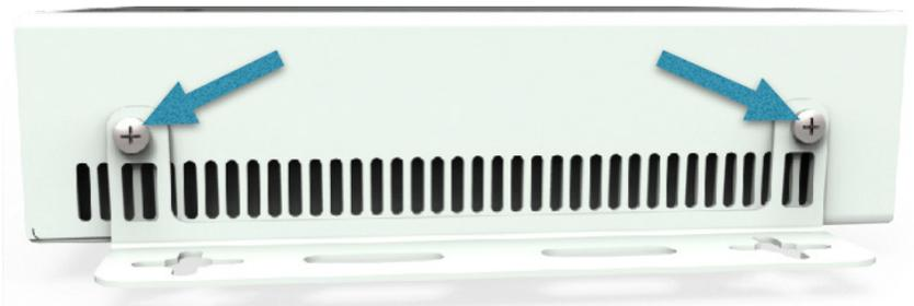
**Sheet Metal Shelf or Equipment:** #6 up to #10 thread-forming or thread-cutting machine screws. Pilot holes should be drilled using the equipment as an outline template. Should the removal of equipment periodically be required use thread-cutting screws. The recommended sequence of hardware would be; Flat Washer, ZyPer4K L-Bracket, Flat washer, Lock Washer (when using thread cutting screw), Screw or Bolt.
