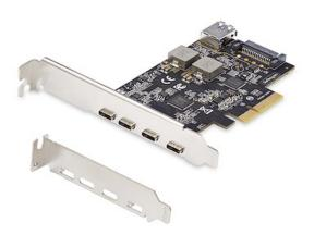
Upgrade or expand a desktop or server's USB connectivity by adding four external USB Type-C 10Gbps ports and one internal USB Type-A 10Gbps port via a single PCI Express x4 connection.
