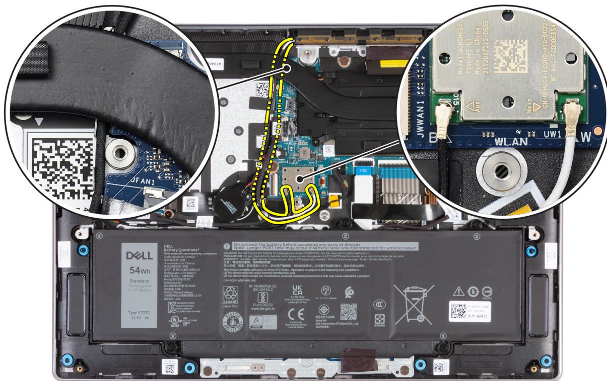
Figure 72. Installing WLAN-antenna cables
