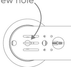
Rotate the camera clockwise to install it.
