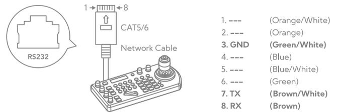
RS232 Serial port connection on controller side.
