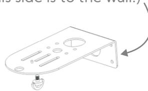
Mounting the bracket vertically to the wall with screws.
