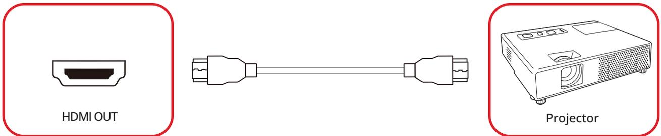
To output video via an external display device, connect an HDMI cable to the **HDMI IN** port of your external display device, and the other end to the **HDMI OUT** port of the display.
