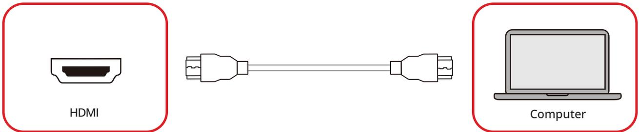
Connect an HDMI cable from your external device to an **HDMI IN** port on the display.
