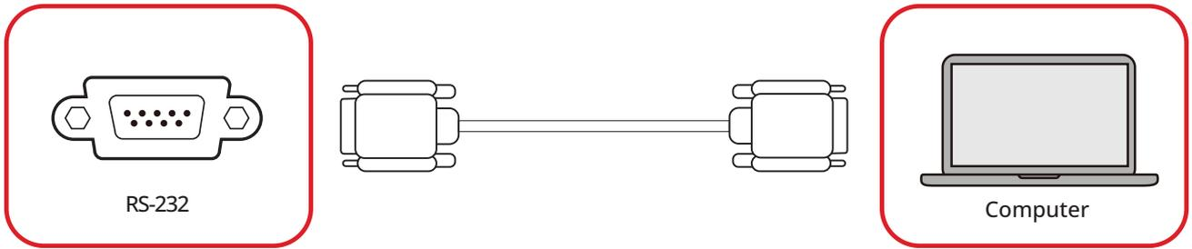
When you use a RS-232 serial cable to connect the display to an external computer or control system, certain functions can be controlled remotely such as: power on and off, volume adjustment, input select, brightness, and more.
