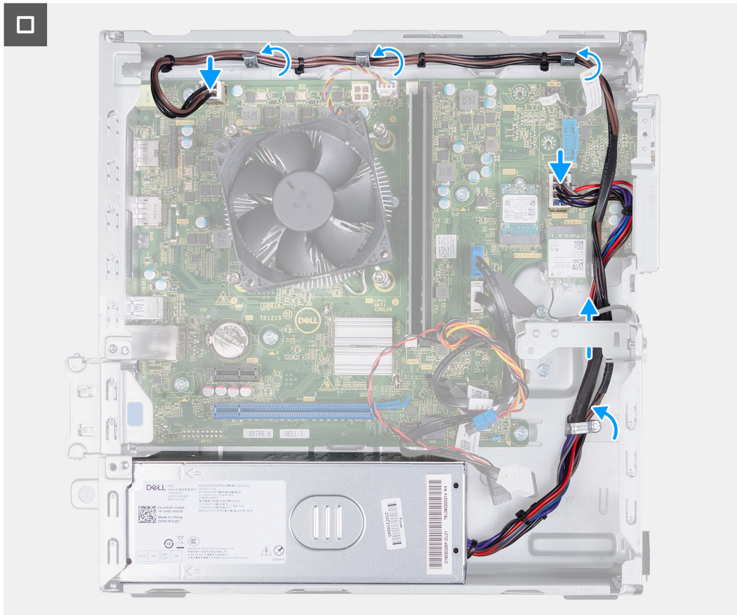
Figure 43. Routing the cables through the routing guides
