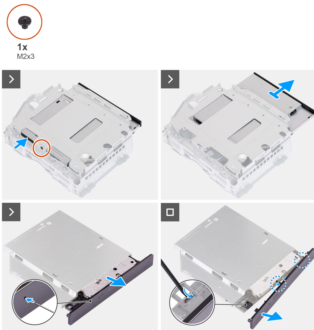
Figure 20. Removing the optical drive
