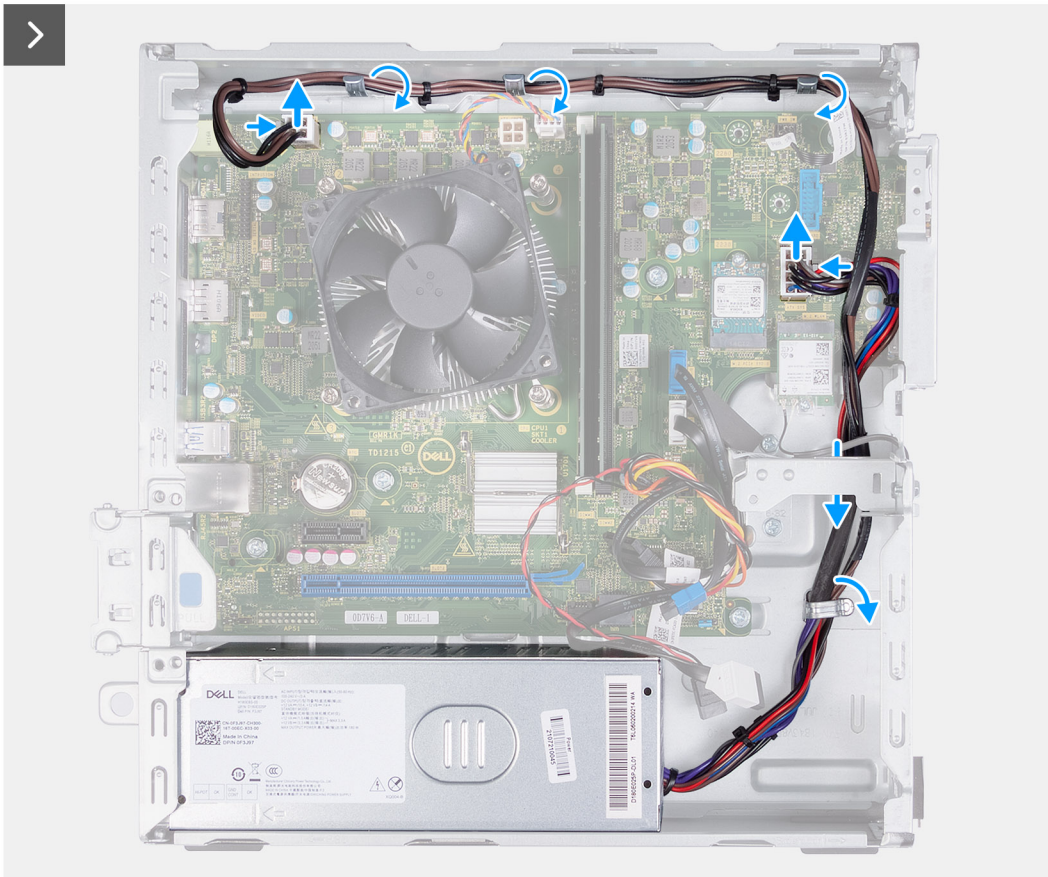
Figure 40. Removing the cables from the routing guides
