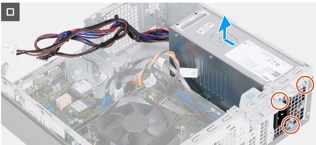
Figure 41. Removing the power supply unit
