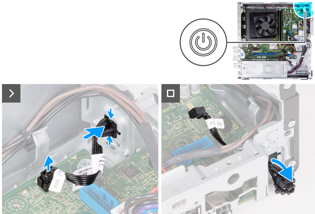
Figure 22. Removing the power button
