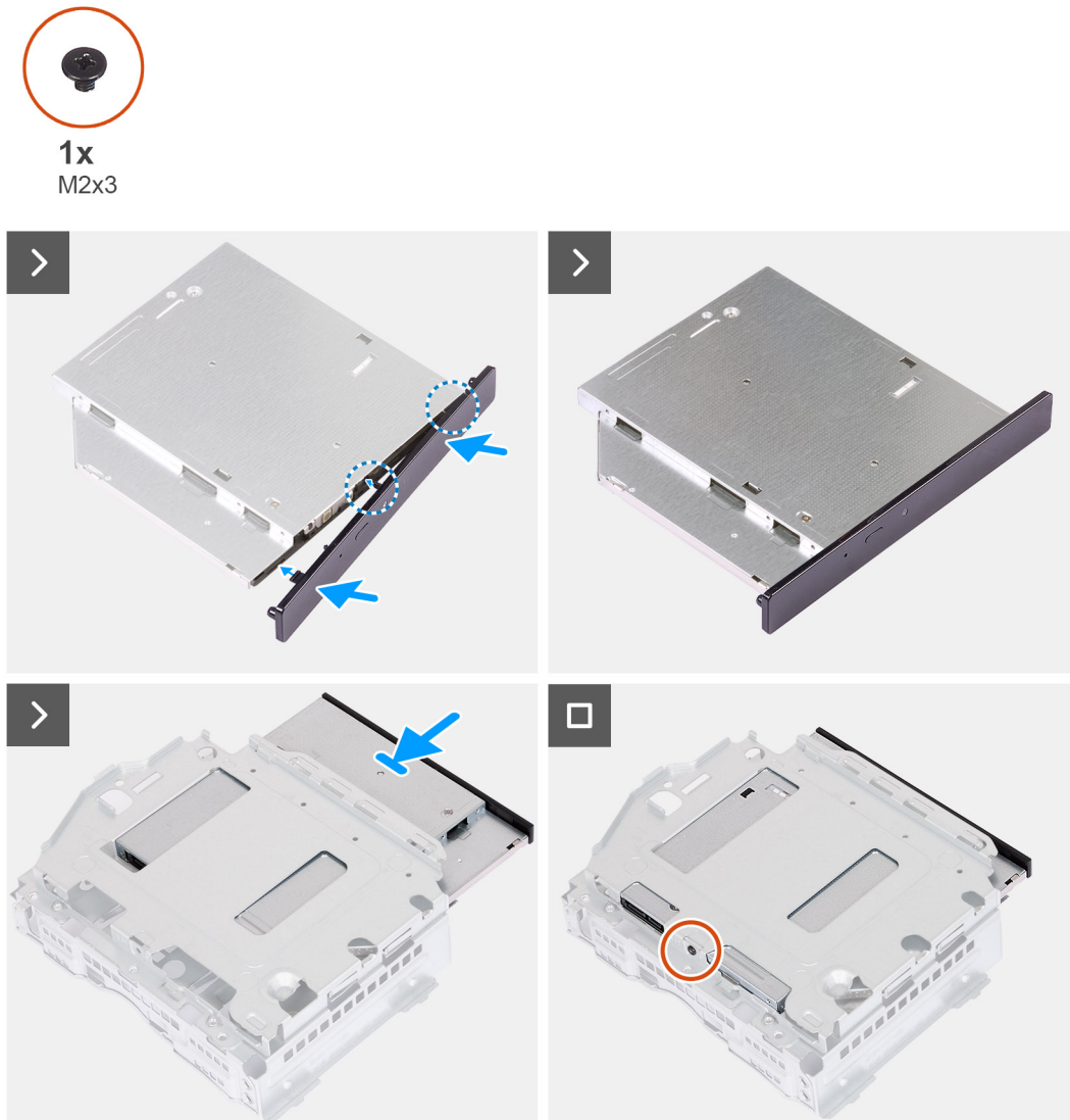
Figure 21. Installing the optical drive
