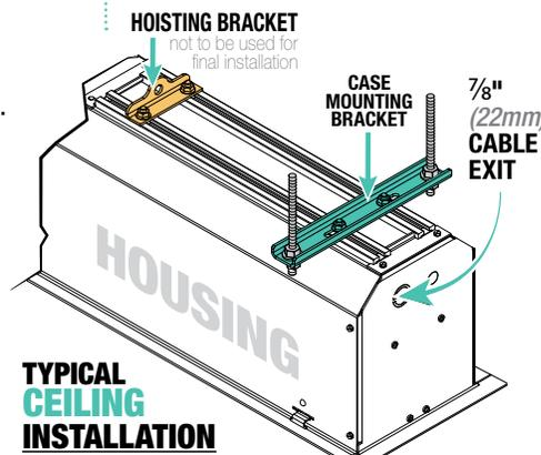
With typical installation, brackets may be angled to meet installation requirements.
