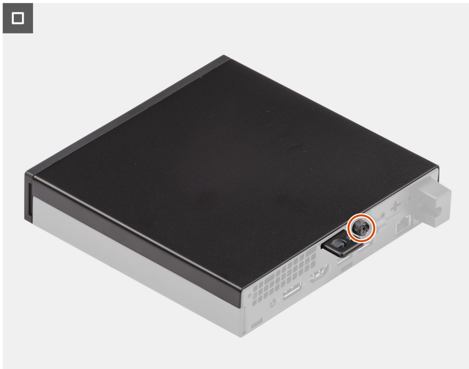
Figure 12. Installing the side cover
