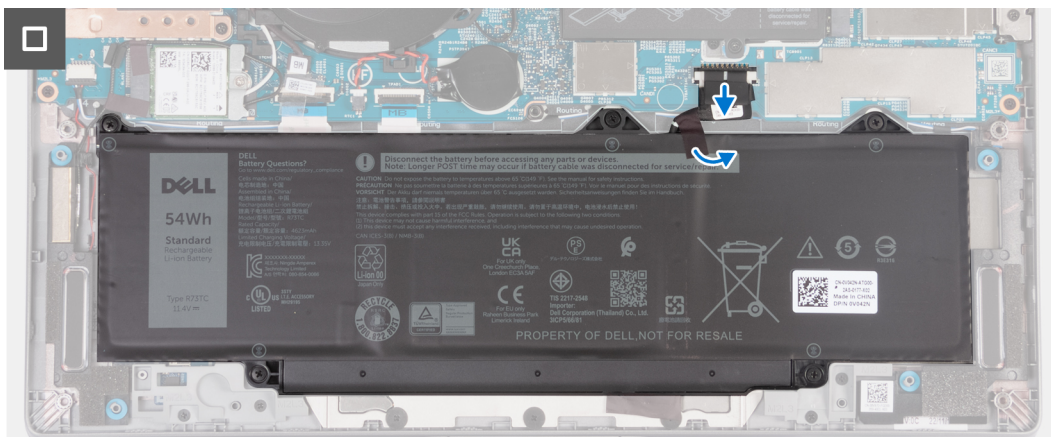
Figure 19. Disconnect the battery cable from the system board
