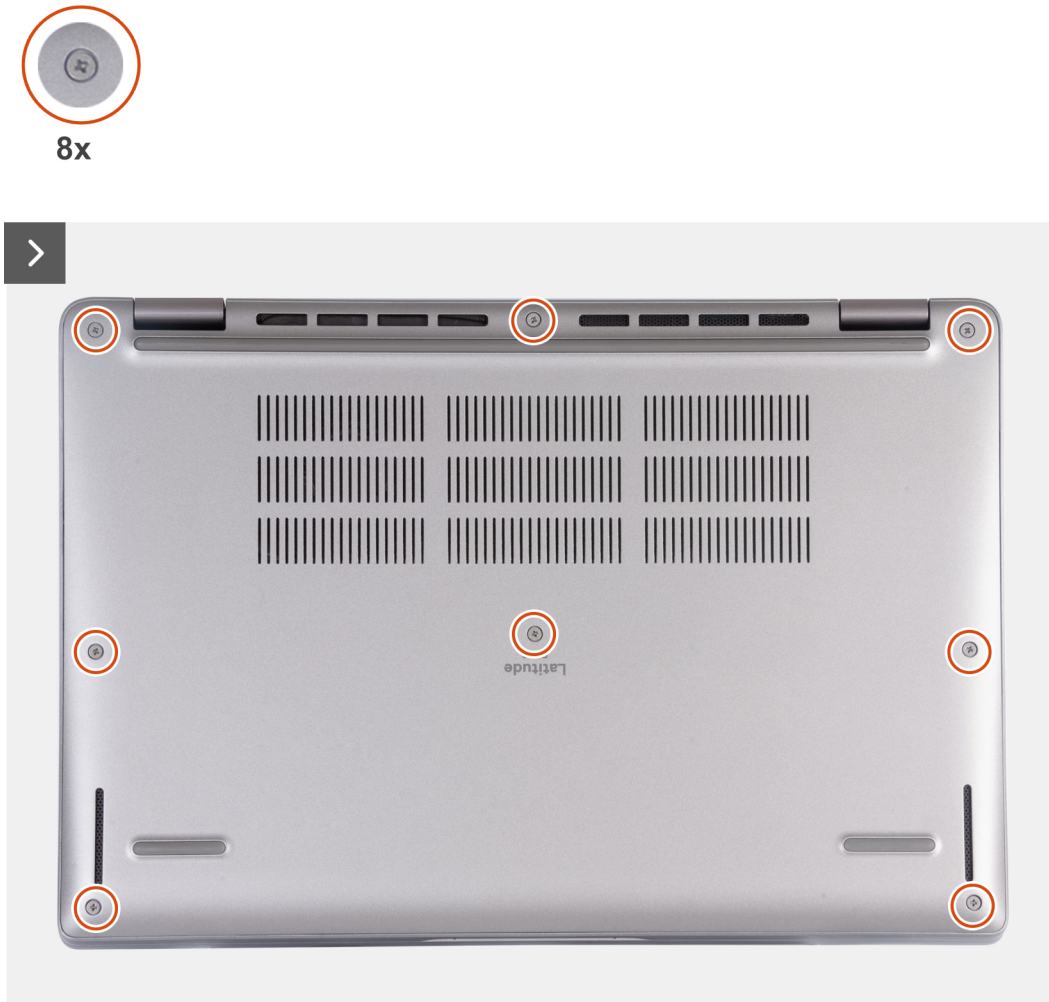
Figure 17. Loosen the eight captive screws that secure the base cover to the palm-rest assembly
