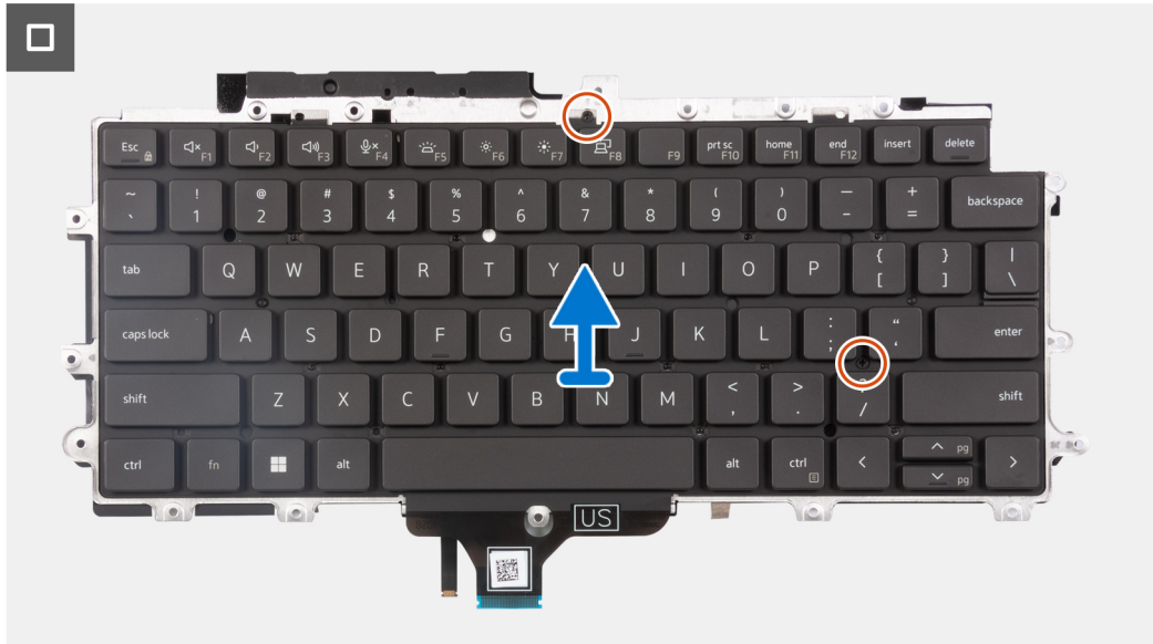
Figure 60. Removing the keyboard assembly
