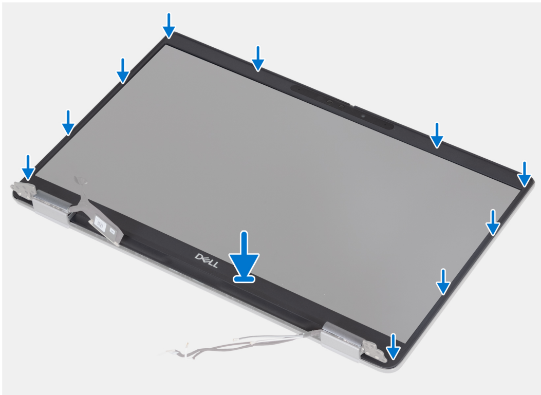
Figure 69. Installing the display bezel (laptop)
