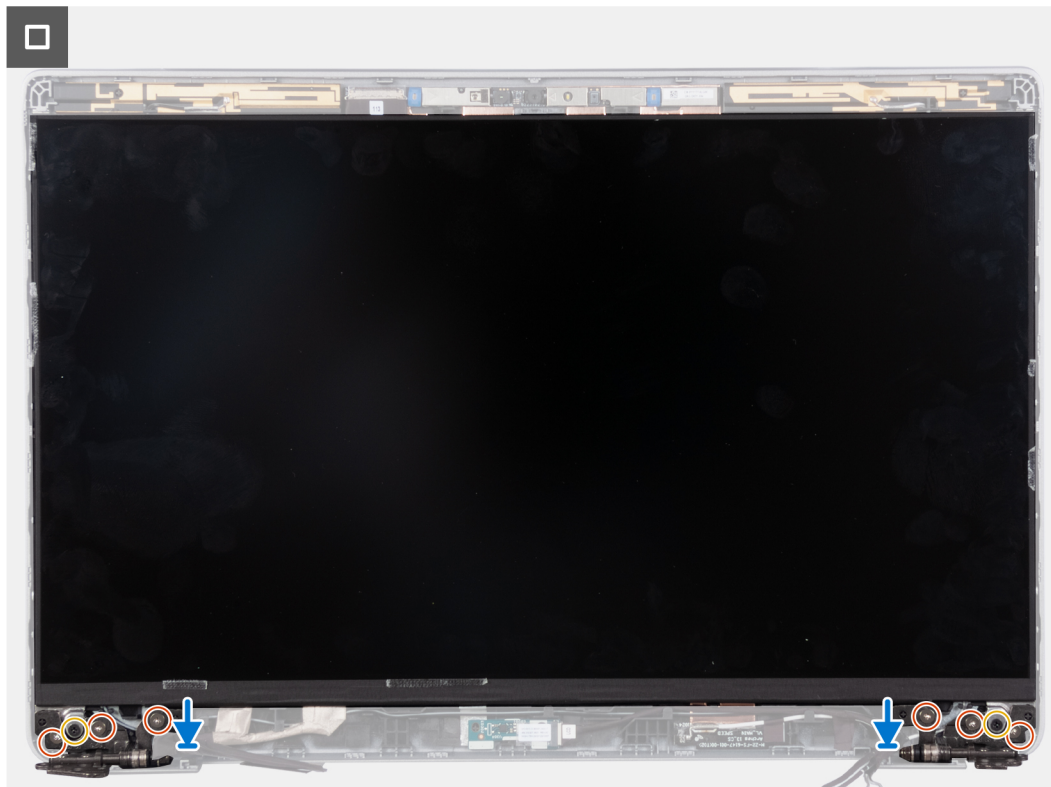
Figure 79. Inserting the display-panel tabs into the slots on the display cover
