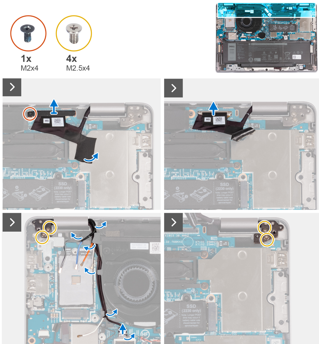
Figure 63. Removing the display assembly
