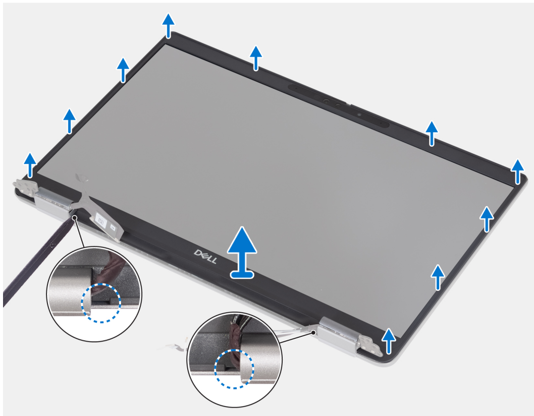
Figure 67. Removing the display bezel (laptop)
