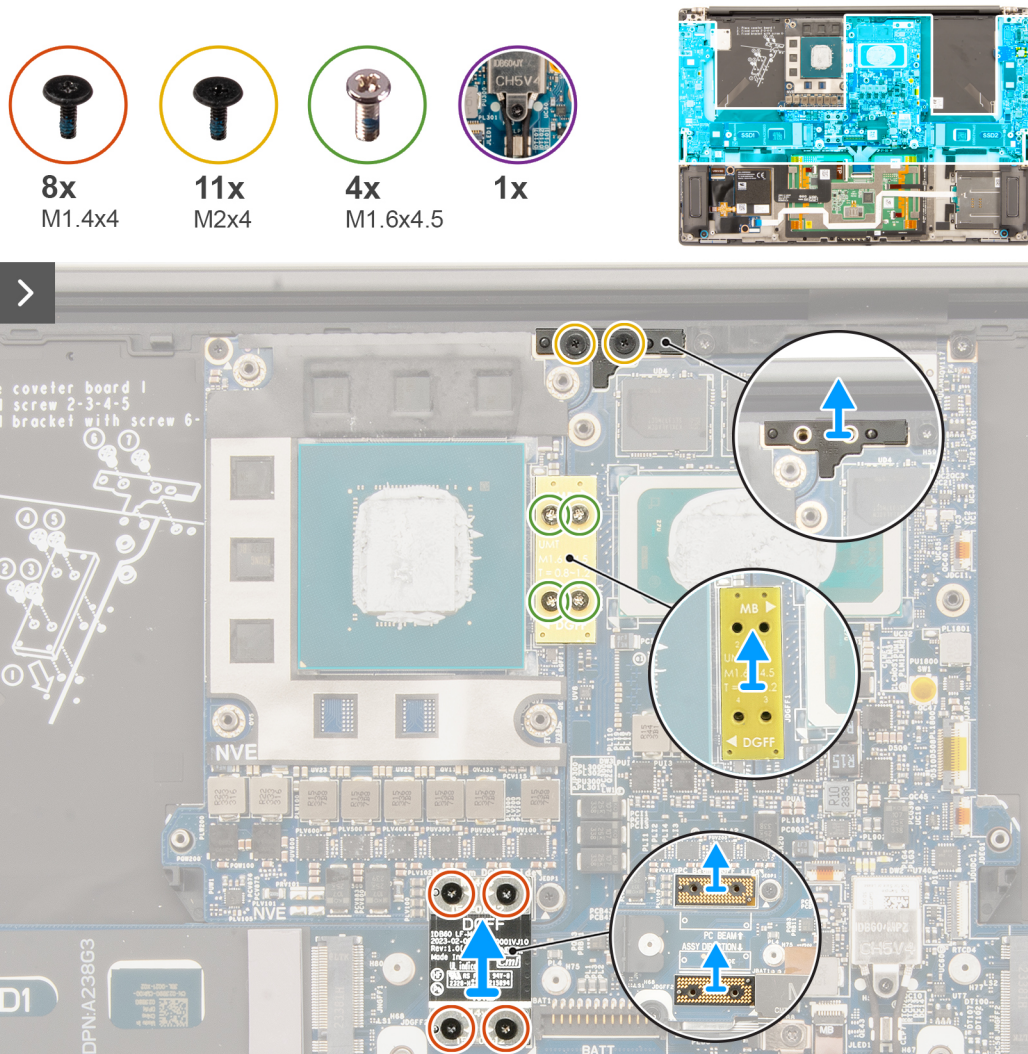
Figure 55. Removing the system board
