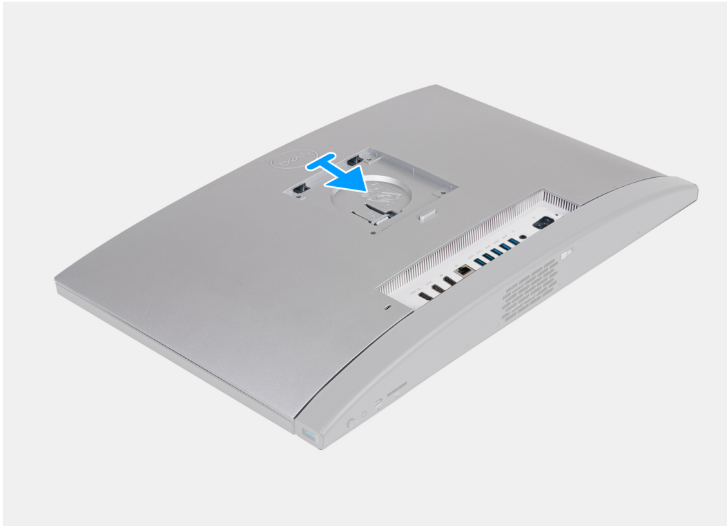
Figure 23. Installing the back cover
