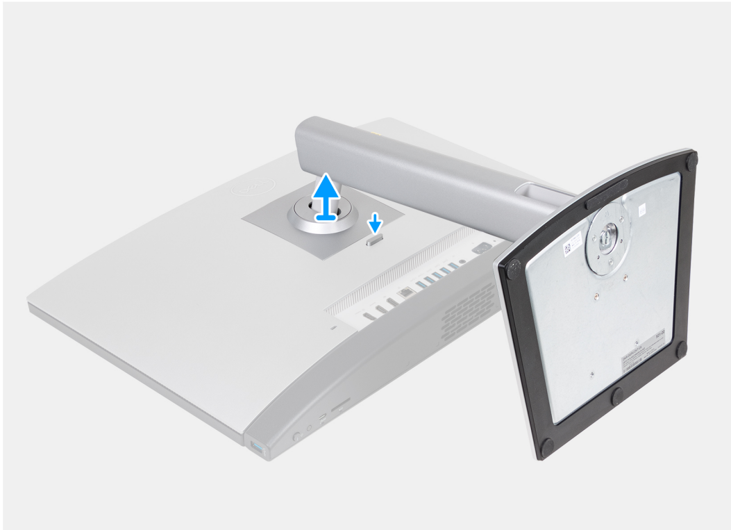
Figure 18. Removing the Height Adjustable Stand (HAS)
