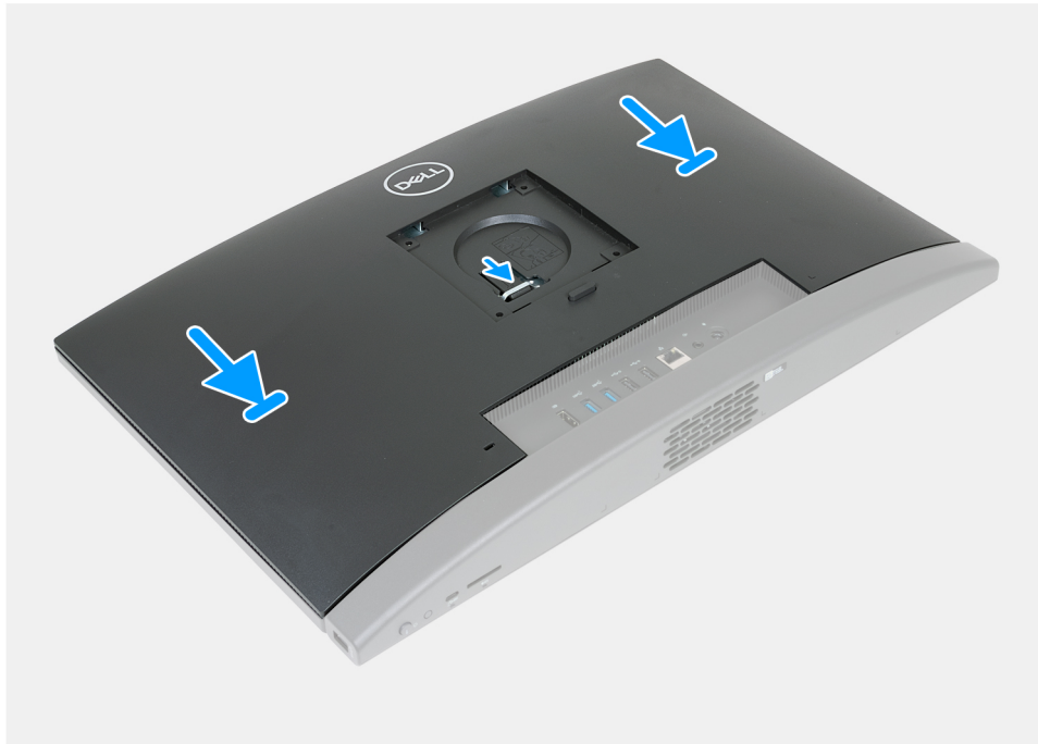
Figure 83. Installing the back cover
