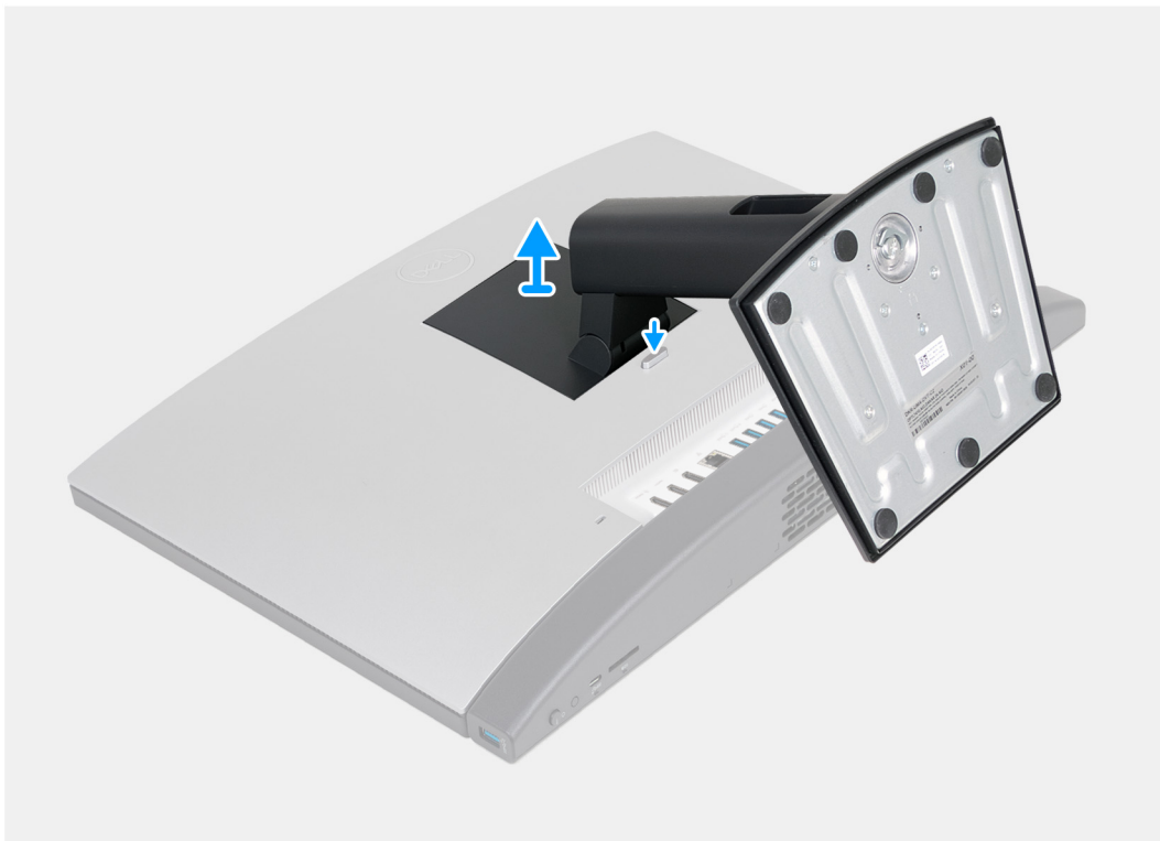
Figure 19. Removing the Fixed Stand
