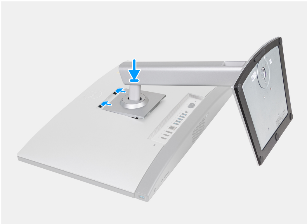
Figure 20. Installing the Height Adjustable Stand (HAS)
