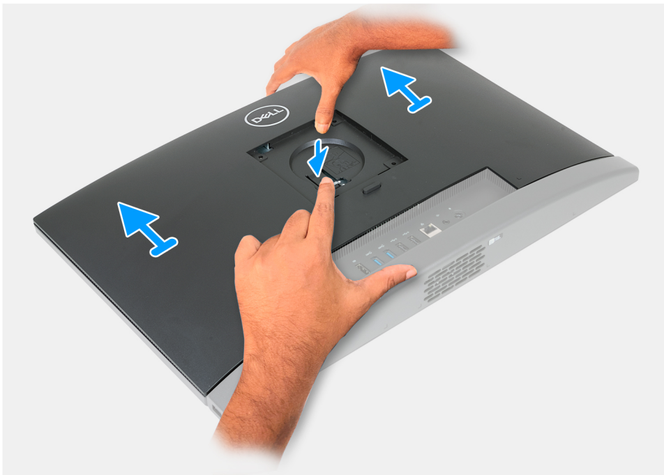
Figure 82. Removing the back cover
