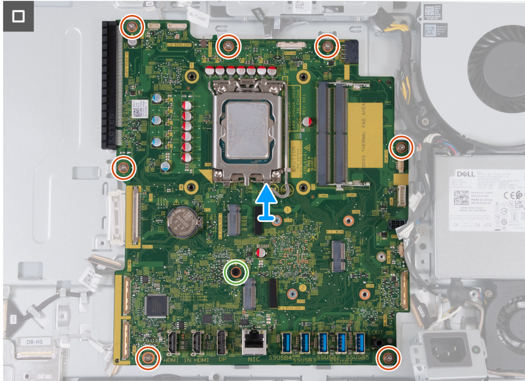
Figure 68. Removing the system board
