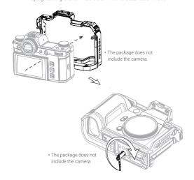
Step 2: • Loosen the locating blocks on both cage sides (do not unscrew the screws completely).
