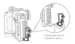
Step 2: Insert the cable and tighten the thumbscrews to secure the cable
